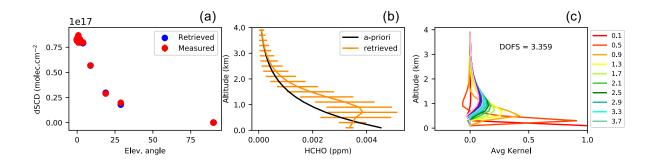
**Figure 3.** Example HEIPRO retrieval from Broadmeadows on 13/12/2017 at 14:00 local time. (a) shows model-measurement dSCD comparison, (b) shows the retrieved and a priori profiles, (c) the averaging kernels for this retrieval.
