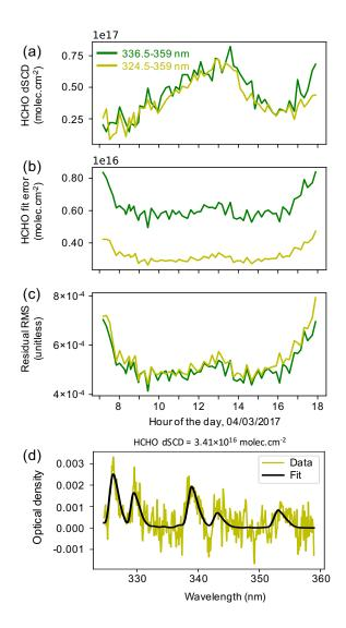
**Figure 2.** (a)-(c) Results of sensitivity tests to determine the appropriate fitting range for formaldehyde, using  $3^{\circ}$  elevation angle data from 04/03/2017 at Broadmeadows, showing dSCD, dSCD fit error and residual RMS respectively. (d) Example  $3^{\circ}$  elevation angle HCHO DOAS fit from 11 am local time on the same day.
