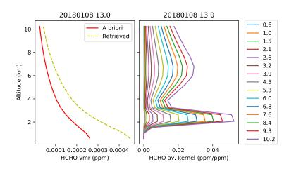
**Figure 4.** Example FTIR profile retrieval from 1 pm local time on 8th January 2018 at Lauder. The left hand panel shows a priori and retrieved HCHO profiles in the lowest 10 km, the right hand panel shows the corresponding averaging kernels.
