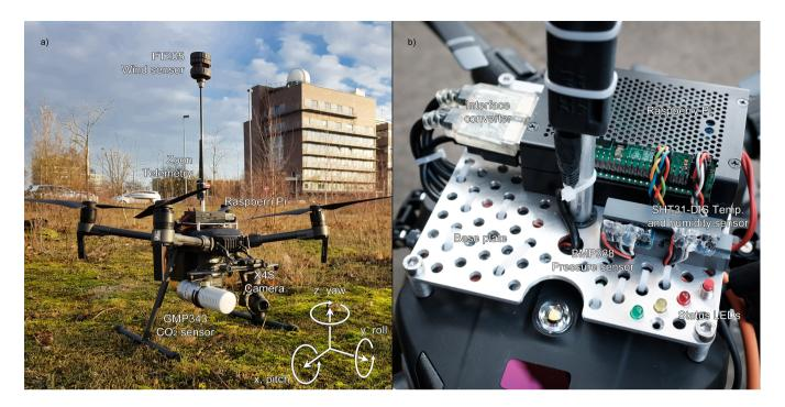
Figure 1. UAV and instrumentation. Left: Overview including UAV coordinate system as defined by us. Right: Zoom on base plate.
