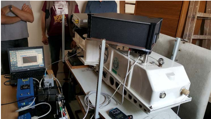
Figure 8: TuPS in-field measurement arrangement (taken during the Dobson calibration in CHMI Hradec Kralove). On right side - TuPS light engine coupled with the Dobson, on bottom left corner - driving PC and fibre-coupled discharge UV broadband radiation source.
