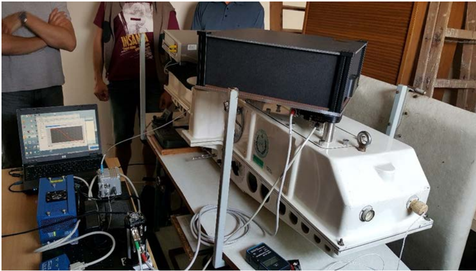
275 Figure 8: TuPS in-field measurement arrangement (taken during the Dobson calibration in CHMI Hradec Kralove). On right side - TuPS light engine coupled with the Dobson, on bottom left corner - driving PC and fibre-coupled discharge UV broadband radiation source.
