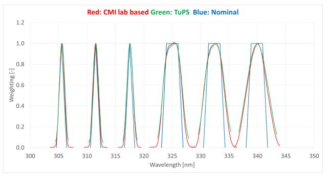
Figure 10: Comparison of in-field calibration and CMI laboratory-based calibration of Dobson #074.
