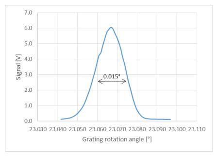
Figure 6: TuPS bandwidth measurement performed at 305 nm. The width of the pike of  $0.015^{\circ}$  corresponds to spectral FWHM 0.12 nm
