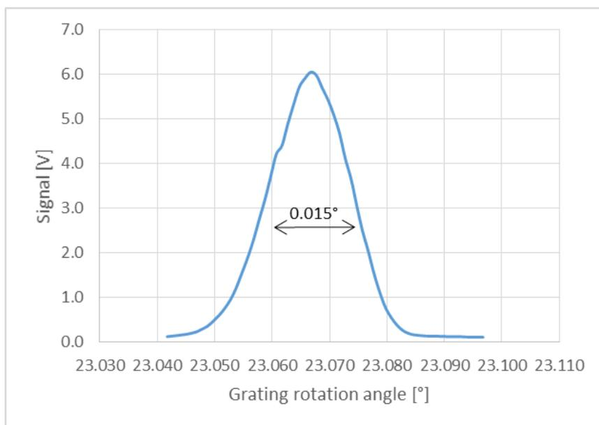
**Figure 6: TuPS bandwidth measurement performed at 305 nm. The width of the pike of 0.015° corresponds to spectral FWHM 0.12 nm**
