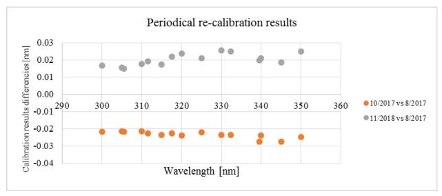
Figure 11: TuPS results of periodical recalibration of the wavelength scale after each in-field measurement.
