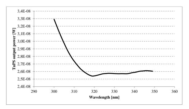
250 Figure 7: Optical power output of TuPS light engine in the spectral region of interest.
