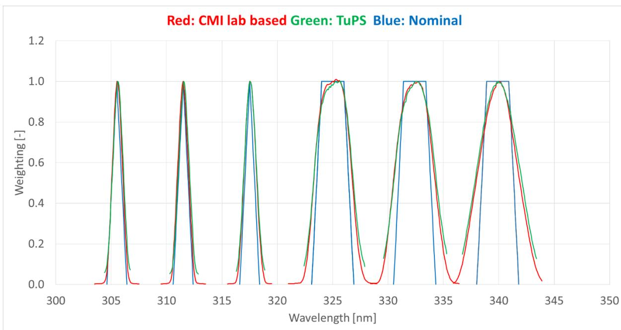
260 Figure 10: Comparison of in-field calibration and CMI laboratory-based calibration of Dobson #074.
