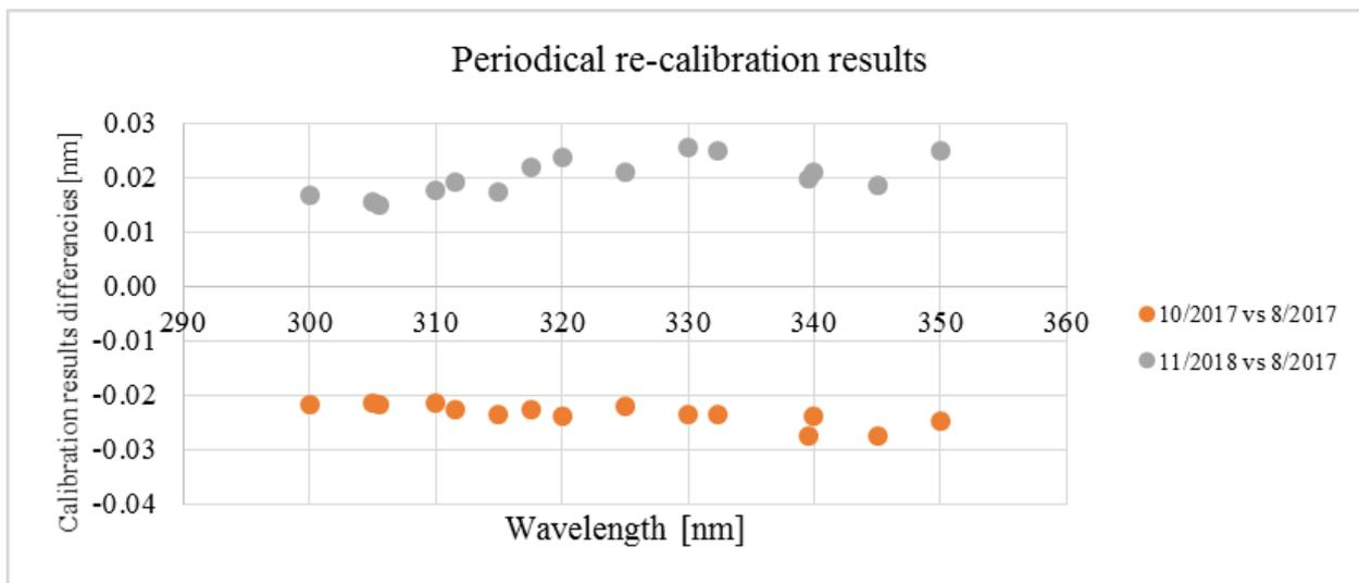
Figure 11: TuPS results of periodical recalibration of the wavelength scale after each in-field measurement.
