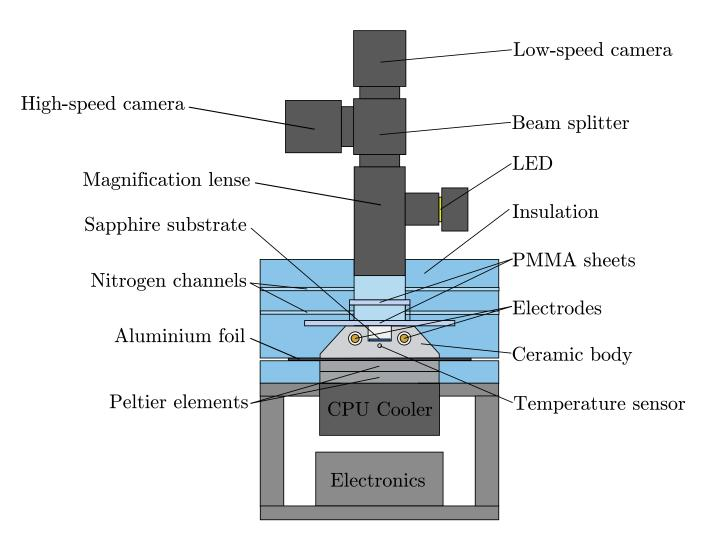
**Figure 2.** Schematic of the experimental setup used for the examination of ice nucleation in a droplet ensemble exposed to an electric field, further extended and republished with permission of SAE International, from Löwe et al. (2019); permission conveyed through Copyright Clearance Center, Inc..
