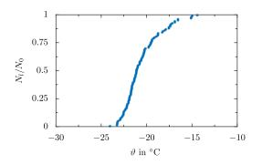
Figure 13. Droplet survival curve for a constant cooling rate of  $\dot{T} = 5$  K/min and without electric field strength, derived through merging the survival curves obtained from several test runs at the respective field strength, resulting in a minimum of 83 droplets per shown survival curve.
