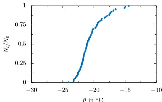
**Figure 13.** Droplet survival curve for a constant cooling rate of  $\dot{T} = 5 \text{ K/min}$  and without electric field strength, derived through merging the survival curves obtained from several test runs at the respective field strength, resulting in a minimum of 83 droplets per shown survival curve.
