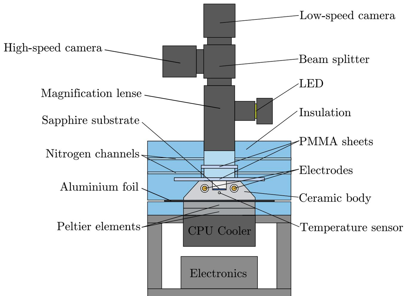
**Figure 2.** Schematic of the experimental setup used for the examination of ice nucleation in a droplet ensemble exposed to an electric field, further extended and republished with permission of SAE International, from Löwe et al. (2019); permission conveyed through Copyright Clearance Center, Inc..
