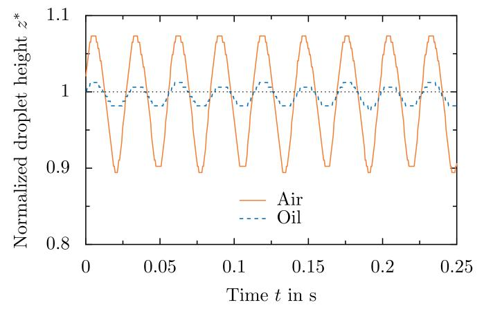
Figure 10. Comparison of droplet oscillation for different surrounding fluids by means of the temporal variation of the normalized height of the droplet. The data corresponds to the droplet shown in Fig. 9.
