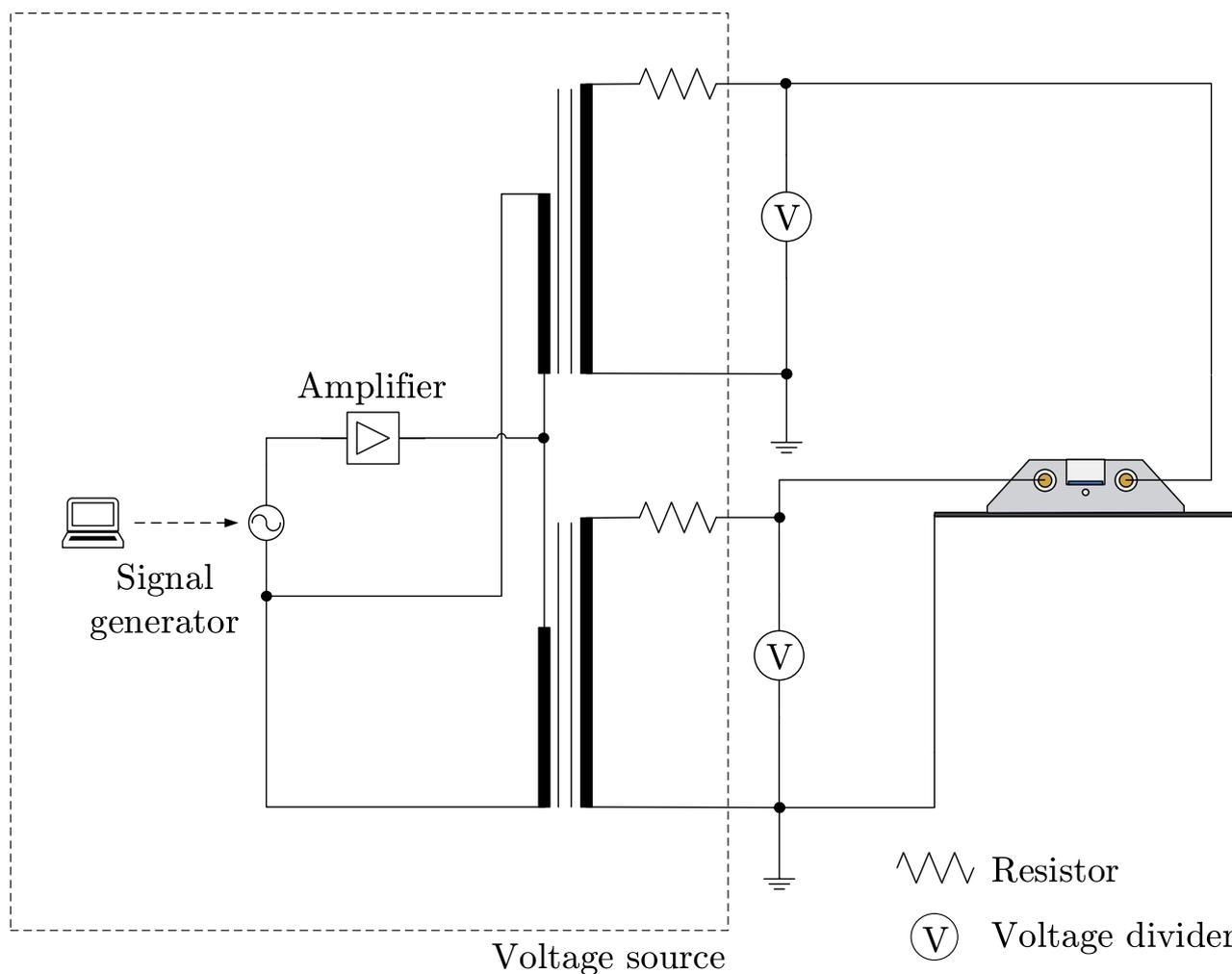
**Figure 5.** Schematic wiring diagram of the system for the power supply used to provide an alternating electric field. The voltage dividers are used to measure the applied voltage. The dashed rectangle represents the voltage source and can be replaced according to the required type of electric field.
