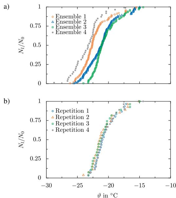
**Figure 12.** Demonstration of the present methodology by means of a comparison of the droplet survival curves obtained from several test runs without an electric field, performed using a) four different droplet ensembles, and b) the same droplet ensemble for each of the four test runs. All data is obtained at  $\dot{T} = 5$  K/min. Republished with permission of SAE International, from Löwe et al. (2019); permission conveyed through Copyright Clearance Center, Inc..
