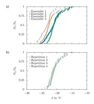
**Figure 12.** Demonstration of the present methodology by means of a comparison of the droplet survival curves obtained from several test runs without an electric field, performed using a) <u>four different</u> droplet ensembles, and b) the <u>same</u> droplet ensemble for each of the four test runs. All data is obtained at  $\dot{T} = 5$  K/min. Republished with permission of SAE International, from Löwe et al. (2019); permission conveyed through Copyright Clearance Center, Inc..
