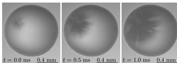
**Figure 7.** Top-view image sequence of dendritic freezing of a sessile supercooled water droplet with  $d = 1.02$  mm (wetted substrate area), captured using a high-speed video camera. Nucleation inside the droplet at a temperature of  $\vartheta = -22.65$  °C is followed by dendritic freezing of the supercooled water droplet. Note that although the shown droplet is not exposed to an electric field, the present experimental setup allows examination of that situation.
