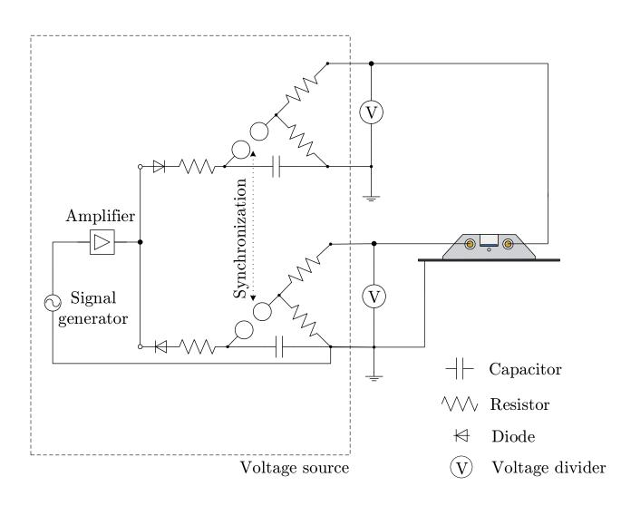
Figure 6. Schematic wiring diagram of the system for power supply used to generate a transient electric field with high initial peak field strength and a continuous decay of the field strength.
