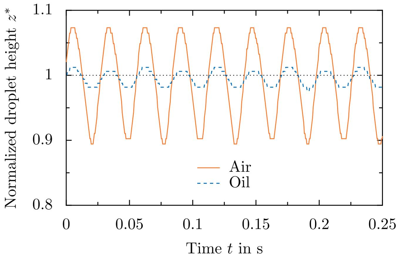
**Figure 10.** Comparison of droplet oscillation for different surrounding fluids by means of the temporal variation of the normalized height of the droplet. The data corresponds to the droplet shown in Fig. 9.
