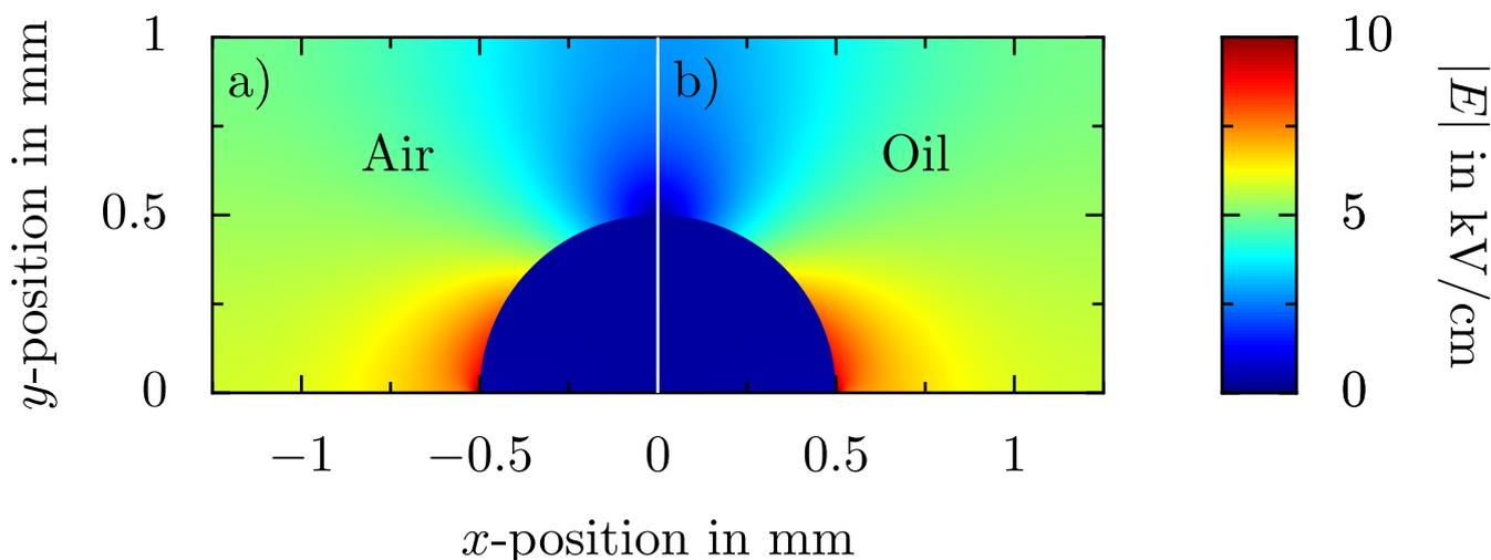
**Figure 11.** Comparison of the electric field distribution for a droplet deposited onto a rigid substrate between two plate electrodes for a) air and b) oil as the surrounding fluid. An alternating voltage of  $U = 10\text{ kV}$  ( $f = 50\text{ Hz}$ ) is applied between the electrodes, resulting in  $\hat{E} = 4\text{ kV/cm}$ .
