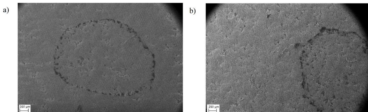
Figure 1. Panel a) Shows Fig.5 b) from manuscript showing 3  $\mu\text{l}$  of PEG-8 with concentration of 0.01  $\text{g L}^{-1}$ . Panel b) shows SEM figure of 3  $\mu\text{l}$  of PEG-8 with concentration of 0.25  $\text{g/l}$  in ACN deposited on the filter.
