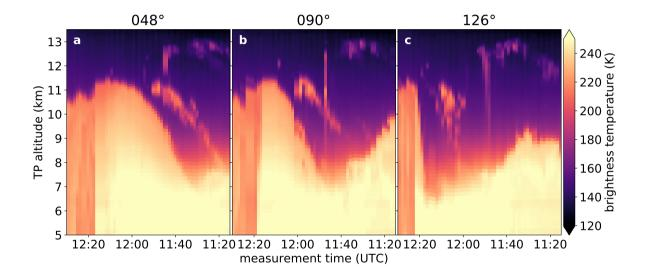
Figure 12. Brightness temperature of GLORIA measurements averaged over the wavenumber range from  $831.2 \text{ cm}^{-1}$  to  $835 \text{ cm}^{-1}$  (the same that is used as in the tomographic retrieval) over time sorted according to azimuth angle in relation to aircraft heading.
