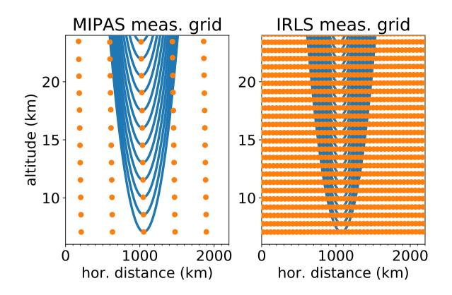
**Figure 1.** The measurement grid of a MIPAS-like instrument (left panel) and the IRLS (right panel). The blue lines indicate the line-of-sights lines-of-sight of a single profile limb-scans. The orange dots indicate the tangent points of multiple adjacent profiles 2100 km along-track.
