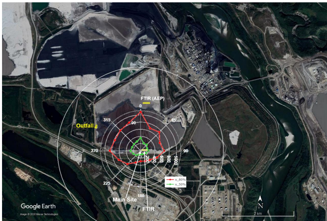
665 Figure 1 Map of the site: FTIR paths are shown as yellow lines (main FTIR on the south shore, AEP FTIR on the north shore), and the outfall is shown as a yellow pin on the west shore. The colored rose plot shows 50% and 80% contribution distances for eddy covariance fluxes at 18m using the Flux Footprint Prediction (FFP) model (Kljun et al. (2015)). Distances are in meters. The large white circle labels the 2.3 km distance from the main site, equivalent to 100 times the height of the highest point of the top FTIR path. This figure is adapted from You et al., (2020) Figure 1.
