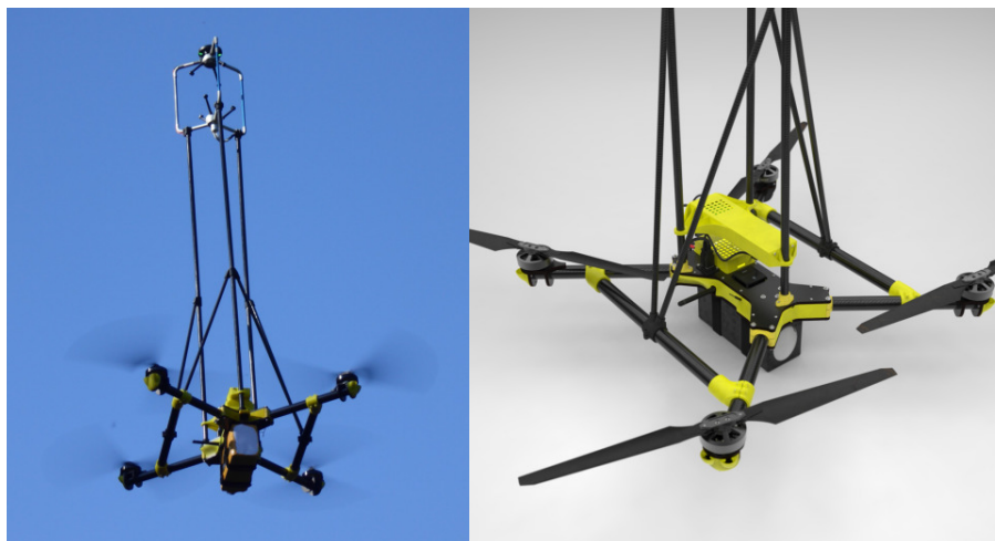
Figure 3. Left: The OPTOkopter drone with a Gill Windmaster on a 1 m long mount during a measurement flight. Right: Rendering of the CAD model.
