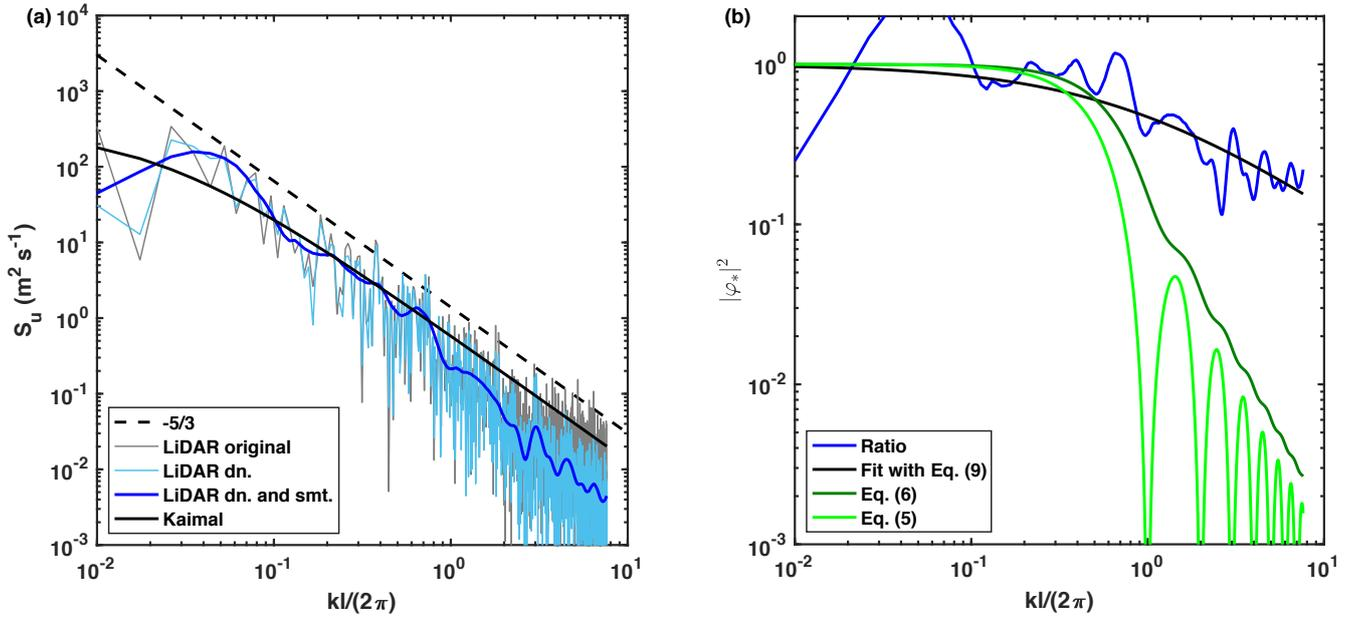
**Figure 4.** Correction of the LiDAR velocity spectrum from the XPIA dataset: (a) velocity spectra of the raw LiDAR data (grey), LiDAR data after application of the de-noising procedure (To et al., 2009) (light blue), LiDAR data after smoothing procedure (dark blue), Kaimal spectrum (black) and  $-5/3$  slope (black dashed); (b)  $|\varphi_*|^2$  (blue),  $|\varphi_*|^2$  fitted with Eq. 9 (black); predictions from Eq. 5 (dark green) and Eq. 6 (bright green) are reported as well.
