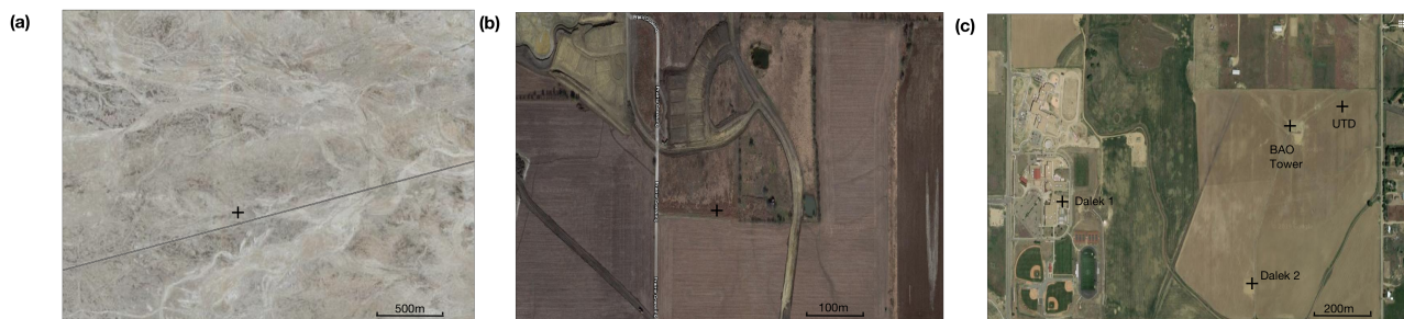
Figure 2. Aerial views of the test sites: (a) SLTEST facility; (b) Celina site; (c) XPIA campaign at the Boulder Atmospheric Observatory. Source of ©Google Earth. Black crosses represent the instrument locations. In (c), each LiDAR is labeled with its respective name.
