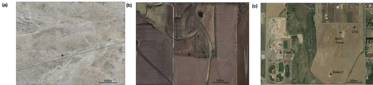
Figure 2. Aerial views of the test sites: (a) SLTEST facility; (b) Celina site; and (c) XPIA campaign at the Boulder Atmospheric Observatory. Source © Google Earth. Black crosses represent the instrument locations. In (c), each lidar is labeled with its respective name.
