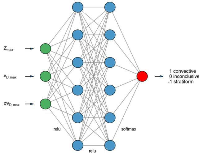
**Figure 6.** Diagram of the neural network with an input layer consisting of three nodes (green) according to the three MRR-based variables, two hidden layers with six nodes each (blue) and the output layer with one node (red).
