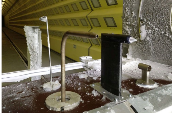
Figure 11. Positioning of the water content probes mounted on the splitter-plate-like panel in the RTA icing wind tunnel test section. Viewing direction is in the direction of flow. From left to right: Cranfield University IKP TW and backward facing BWV inlet, PA hygrometer IKP and SEA WCM-2000.
