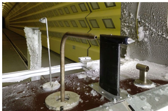
Figure 10. Positioning of the water content probes mounted on the splitter-plate-like panel in the RTA icing wind tunnel test section. Viewing direction is in the direction of flow. From left to right: Cranfield University IKP TW and backward facing BWV inlet, PA hygrometer IKP and SEA WCM-2000.
