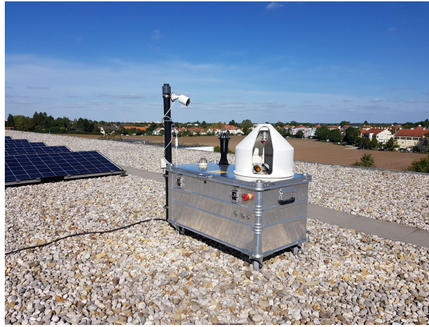
Figure 5. Image of the new enclosure system on the roof of a school at our southern site Taufkirchen. The systems includes, inter alia, the newly designed rotating cover, the lightweight aluminum case, the solar radiation sensor and a surveillance camera attached to a post.
