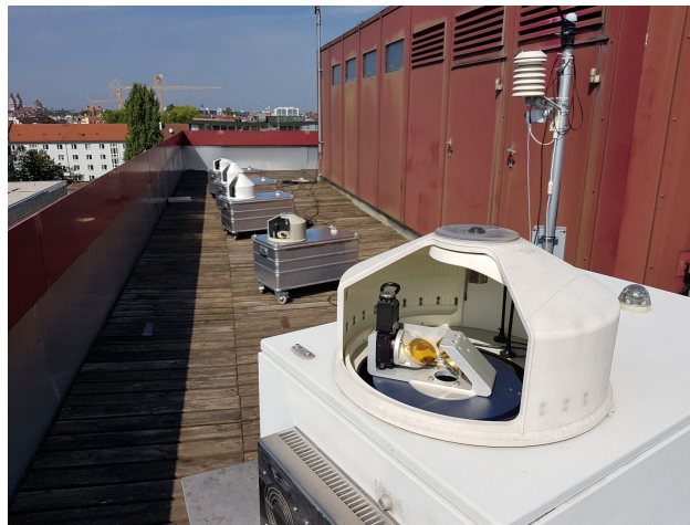
Figure 10. Calibration measurements of all our five sensor systems on top the roof of our institute's building. One can see four slightly different versions of our enclosure systems.
