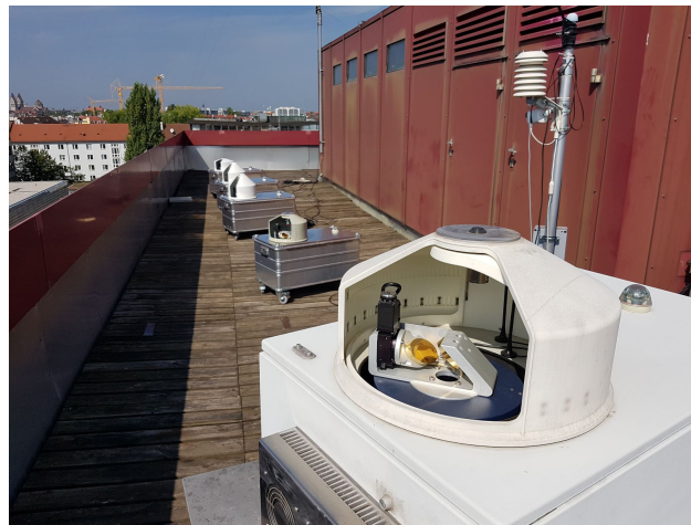
Figure 10. Calibration measurements of all our five sensor systems on the roof of our institute's building. One can see four slightly different versions of our enclosure systems.
