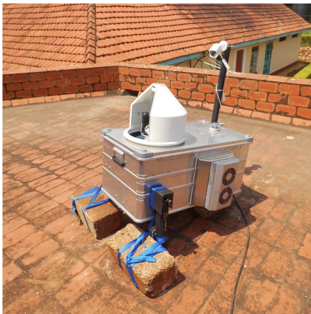
Figure 6. Setup of the tropical version of our enclosure in Jinja, Uganda (Latitude: 0.4^{\circ} N). With the help of car jacks the whole system is tilted in order to enable measurements at high elevation levels close to 90^{\circ} . Furthermore, the system is equipped with two 150 W thermo-electrical coolers (attached at the two sides of the system) that keep the temperature inside the enclosure constant at 25^{\circ}\text{C} .
