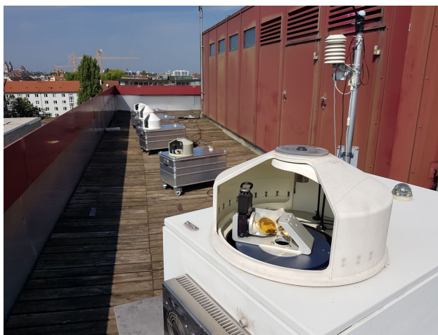
Figure 10. Calibration measurements of all our five sensor systems on top of our institute's building. One can see four slightly different versions of our enclosure systems.
