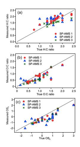
**Fig. 4.** Comparisons between the measured and true values of H:C, O:C, and OS<sub>c</sub> determined by the three SP-AMS using the LV scheme. The I-A method was used for the elemental analysis. Red circles, blue triangles, and green crosses represent data measured by SP-AMS 1, 2 and 3, respectively. The dashed lines represent 1:1 line.
