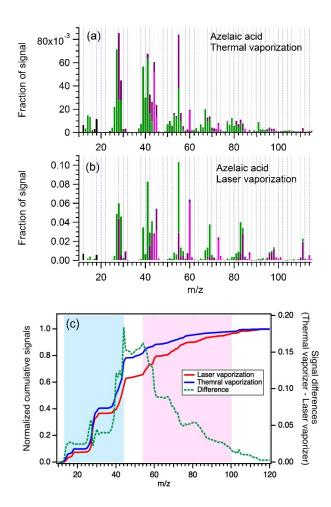
**Fig. 2.** Mass spectra of azelaic acid, measured by SP-AMS 1 using the thermal (a) and laser (b) vaporization schemes. (c) Normalized cumulative histogram of mass-to-charge ratios for the oxygenated organic compounds measured by the SP-AMS 1. The blue area indicates that the thermal vaporization scheme tends to provide organic fragments with
