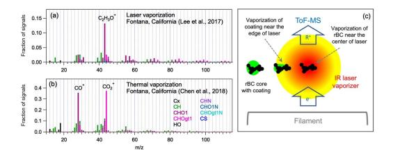
Fig. 1. Mass spectra of more-oxidized OOA materials measured in Fontana, California, using the (a) laser and (b)
