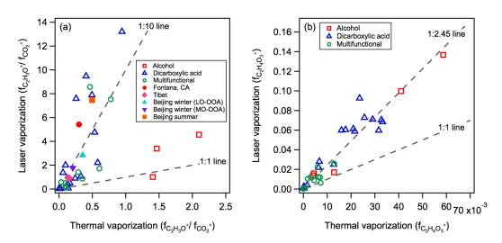
**Fig. 3.** Comparison of (a)  $f_{C_2H_3O^+}/f_{CO_2^+}$  ratios and (b)  $f_{C_2H_4O_2^+}$  measured by the LV and TV schemes from laboratory data (hollow markers) and collocated field measurement (solid markers) (see Table S1 for the detail of ambient data comparison).
