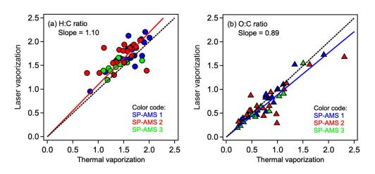
**Fig. 5.** Comparisons of H:C and O:C ratios of oxygenated organic compounds determined by the LV and TV schemes. The I-A method was used for the elemental analysis. The dashed and solid lines represent 1:1 line and data fitting, respectively.
