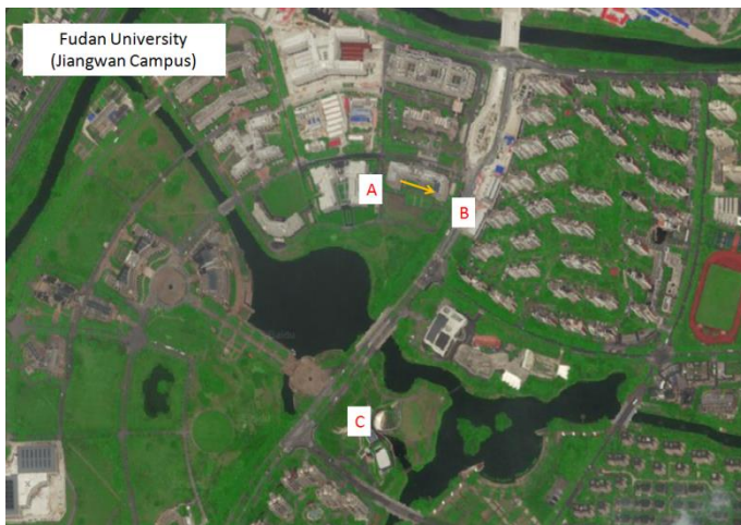
160 161 Figure 5. Field measurement sites of DOAS and on-line VOCs, A is the transmitting telescope, B is the receiving telescope, 162 and C is the on-line VOCs, the yellow arrow is the light path of DOAS. This map is sourced from © Baidu
