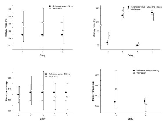
Figure 2: Verification results of the mercury amount (ng) determined on the sorbent tubes during the second comparison. The error bars indicate the expanded uncertainty for the reference value (ng) (k = 2) and the verification value (ng) (k = 2).
