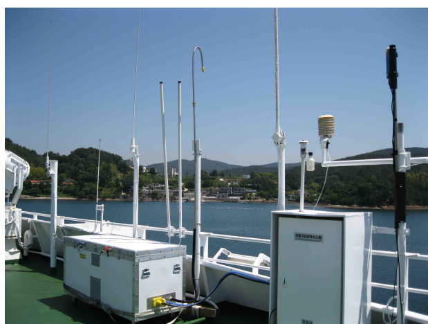
Figure S1. R/V Onnuri (top photo); instruments housed in custom-built box sited along the starboard rail above the bridge (long box, left half of bottom left photo, with tall curved sampling mast just to its right); pumps housed in a separate box located a few meters away along the stern rail (bottom right photo).
