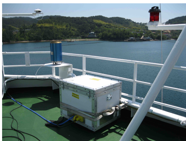
Figure S1. R/V Onnuri (top photo); instruments housed in custom-built box sited along the starboard rail above the bridge (long box, left half of bottom left photo, with tall curved sampling mast just to its right); pumps housed in a separate box located a few meters away along the stern rail (bottom right photo).
