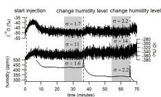
Figure 4: Records of  $\delta^{18}O$ ,  $\delta^{10}D$  and humidity over 3 humidity plateaus (72 ppmv on the left, 425 and 335 ppmv on the right) obtained with the LHLG (December 2018 at Concordia). The grey rectangles indicate the period (10 min) over which the average values are kept for calibrating the data generated by the L2130-i analyzer.
