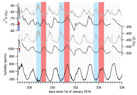
**Figure 7**: Focus on diurnal variability of  $\mathcal{S}^{18}O$ ,  $\partial D$  and humidity recorded at Concordia. Grey curves show the raw measurements and black curves the corrected records. The red (blue) bars indicate the calculated uncertainty due to the isotopes vs humidity dependence (Figure 5) on the corrected  $\mathcal{S}^{18}O$  and  $\partial D$  values during periods with maximum (minimum) humidity. The red (blue) rectangles indicate half day with maximum (minimum) humidity.
