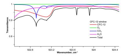
Figure A2. Absorption by various gases in the spectral region of CFC-12 absorption band 1160  $cm^{-1}$ . 19 June 2017, 10:25, solar zenith angle 37°
