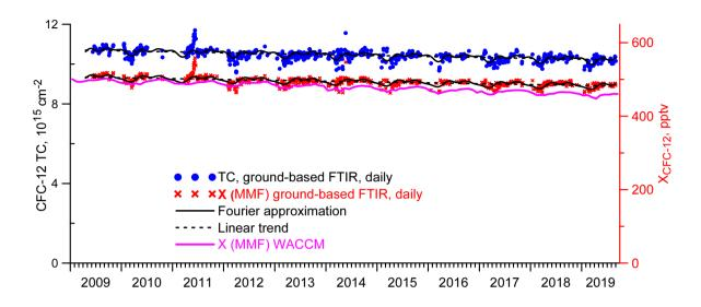
**Figure 5.** Daily mean TCs and Xgas of CFC-12. Filtered results, T-Ph parameter  $\alpha$ =85.
