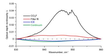
**Figure 2.** Nonlinearity of optical depth components  $\Delta = \tau(\nu) - (\tau_{830} + (\tau_{860} - \tau_{830})(\nu - 830)/30)$ . 29 July 2018, solar zenith angle = 60°.
