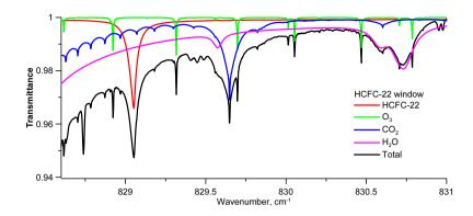
Figure A3. Absorption by various gases in the spectral region near of HCFC-22 absorption line  $829cm^{-1}$ . 19 June 2017, 10:25, solar zenith angle  $37^{\circ}$
