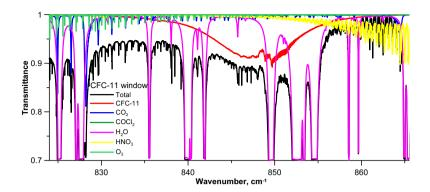
Figure A1. Absorption by various gases in the spectral region of CFC-11 absorption band. 7 November 2017, 09:57, solar zenith angle 76°
