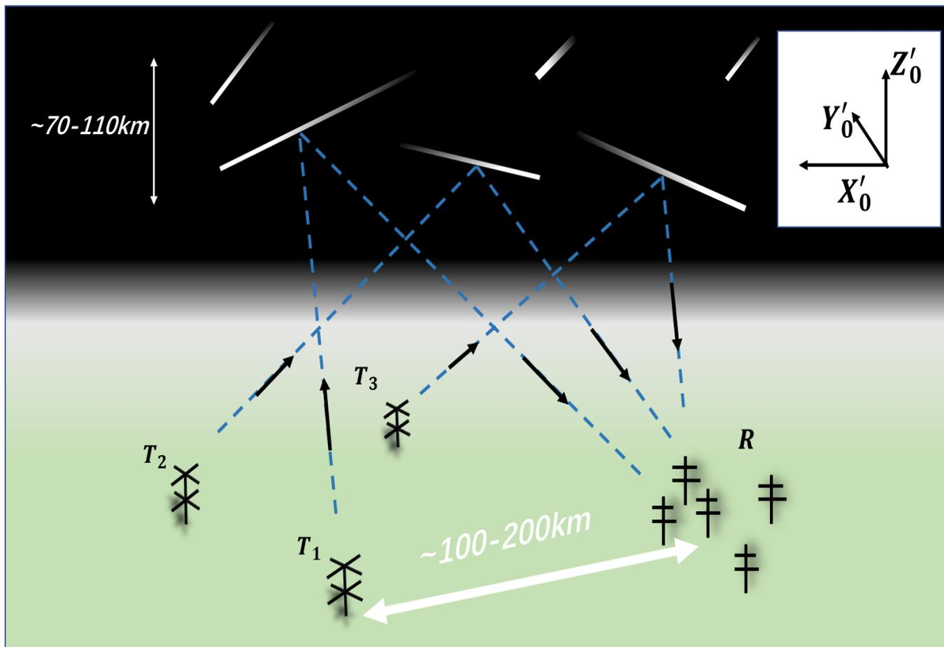
Figure 2: Schematic diagram of the multistatic meteor radar system. There are three transmitters ( $T_1, T_2$  and  $T_3$ ) and one receiver ( $R$ ) in the picture. The distance between the transmitter and receiver is usually approximately 100-200 km.  $X'_0, Y'_0, Z'_0$  represents the west, north and up directions in the receiver.
