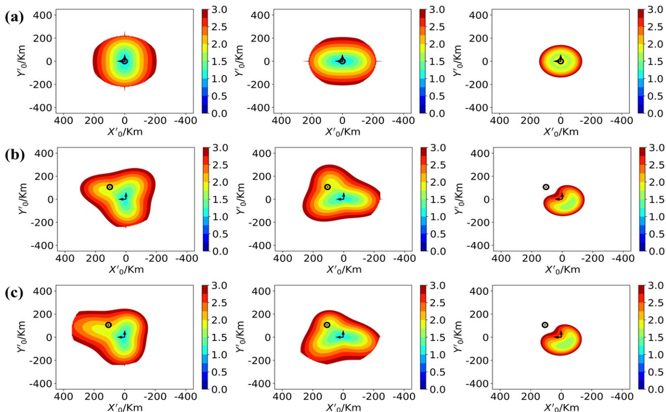
**Figure 8:** Normalized three-dimensional spatial resolution distributions in three-dimensional space with three different settings. (a)  $d = 0$ , monostatic meteor radar (b)  $d = 150\text{ km}$ ,  $\psi_x^{X,i} = \psi_y^{Y,i} = 0$  (c)  $d = 150\text{ km}$ ,  $\psi_x^{X,i} = \psi_y^{Y,i} = 5^\circ$ . Each row from left to right are the resolution distributions in the  $X'_0, Y'_0, Z'_0$  direction, respectively.
