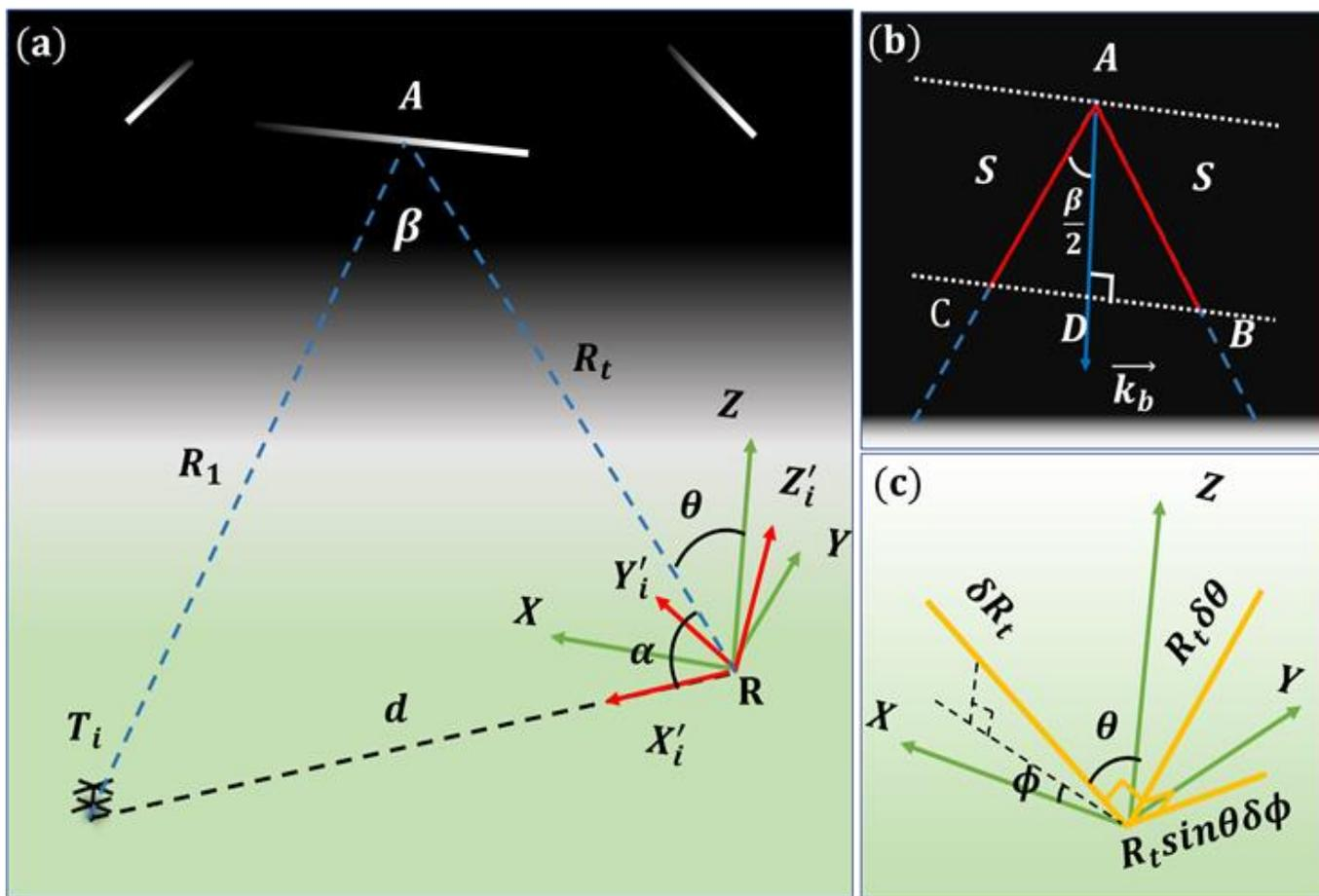
505 Figure 4: (a) Schematic diagram of a forward scatter geometry for the radar link between  $T_i$  and  $R$ .  $A$  is the meteor trail reflection point. (b) Magnified plot of reflection point  $A$ . The red line represents one radio wave pulse, and  $S$  is the half pulse length.  $\vec{k}_b$  is the Bragg vector and halves forward scatter angle  $\beta$ . (c) Schematic diagram of  $E_1$  in  $XYZ$ , which can be decomposed into three orthogonal vectors.
