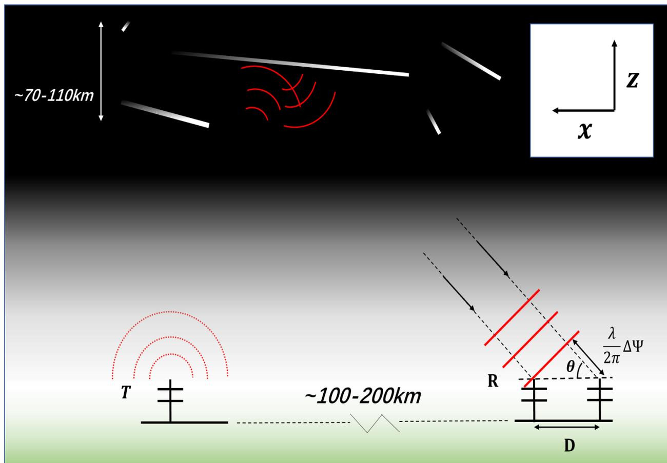
**Figure 1:** Schematic diagram of the bistatic configuration in the HM. The two receiver antennas and the transmitter antenna are collinear. The analysis is in a 2-dimensional vertical plane through the baseline.
