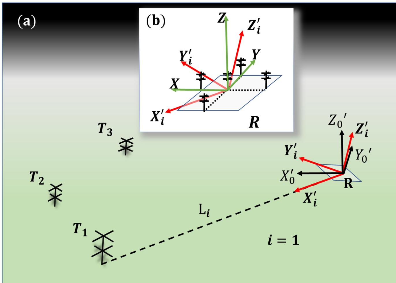
Figure 3: (a) Schematic diagram of three coordinate systems.  $X'_iY'_iZ'_i$  are a class of coordinate systems. In this picture,  $i$  can be 1,2,3. (b) Magnified plot of the receiver.  $XYZ$  is fixed on the receiver horizontal plane. Axis- $X$  and  $Y$  are collinear to two antenna arrays.
