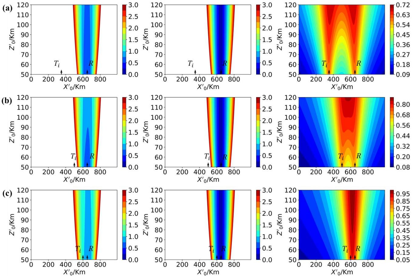
520 **Figure 5:** Two-dimensional space normalized vertical spatial resolution distribution ignoring the error term “ $\delta R_t$ ” (corresponding
