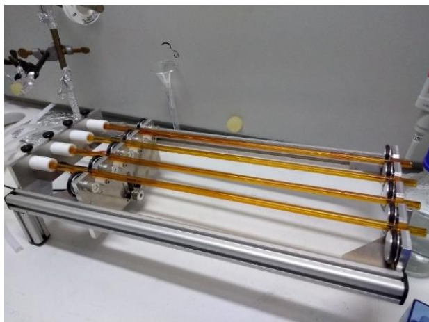
Figure S2: Created system (called “Denudermaster”) for the simultaneous coating of four denuders.
