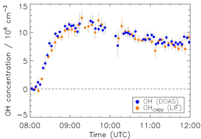
**Figure 4.** Time series of OH concentrations measured by DOAS and LIF (with CMR) in humidified synthetic air in the SAPHIR chamber. The measured OH reactivity in the chamber air was less than  $2 \text{ s}^{-1}$ . The chamber was illuminated by solar radiation and OH was mainly produced by solar photolysis of traces of nitrous acid emitted from the chamber walls. The shown data are averaged over 300 s.
