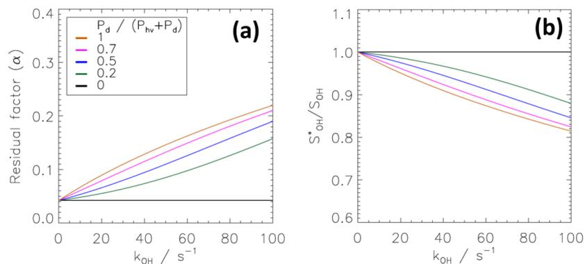
**Figure 8.** Calculated  $k_{OH}$  dependence of the residual factor  $\alpha$  and ratio  $S^*_{OH} / S_{OH}$  using a model that takes inhomogeneous mixing of the scavenger into account (see Section 4.3). The dependence is shown for different ratios of dark to total atmospheric OH production rates. The colored horizontal lines denote the same ratios of dark to total OH production rates as used in Fig. 7.
