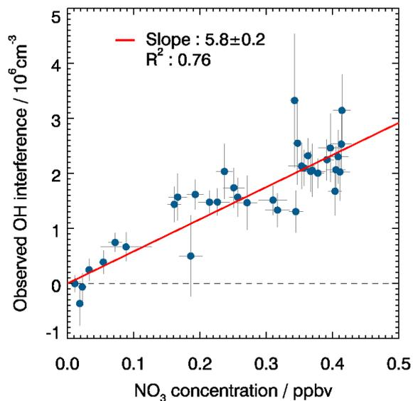
**Figure 6.** Correlation between the measured OH interference, determined by chemical modulation, and the NO<sub>3</sub> concentration measured during an experiment when NO<sub>3</sub> (from thermal decomposition of frozen N<sub>2</sub>O<sub>5</sub> crystals) was present in the chamber. Measurements were fitted to a linear function forced through the origin.
