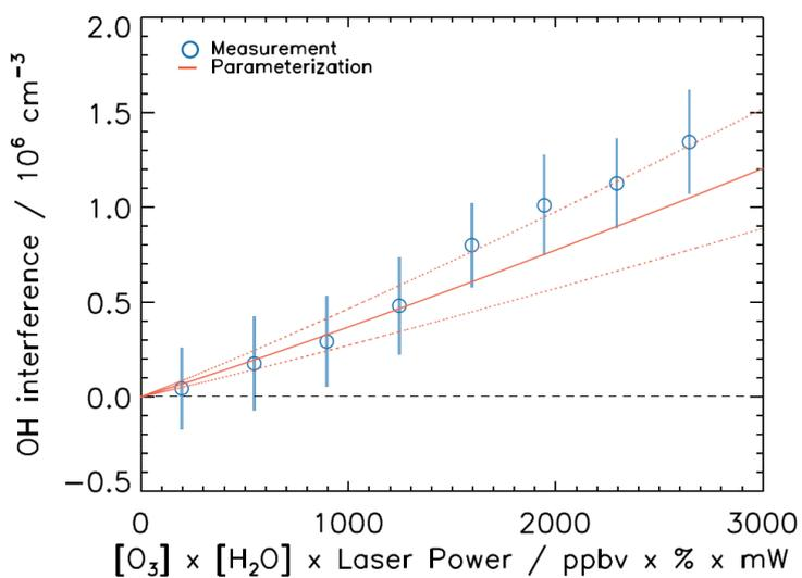
**Figure 13.** Averaged OH interference measured during all JULIAC periods (error bars are  $1\sigma$  errors) compared a parameterization determined in laboratory experiments. The red dotted lines represent the uncertainty of the parameterization.
