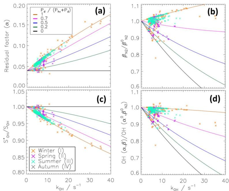
**Figure 10.** Modelled  $k_{\text{OH}}$  dependence of the CMR properties for the atmospheric chemical conditions during the JULIAC periods in different seasons of 2019. Here, the model for a homogeneously mixed scavenger was applied. See Fig. 7 for further explanations of (a) - (c). Panel (d) shows the ratio of corrected to uncorrected ambient OH concentrations, if the  $k_{\text{OH}}$  dependence of  $\alpha$  and  $\beta_{\text{N}_2}$  is taken into account.
