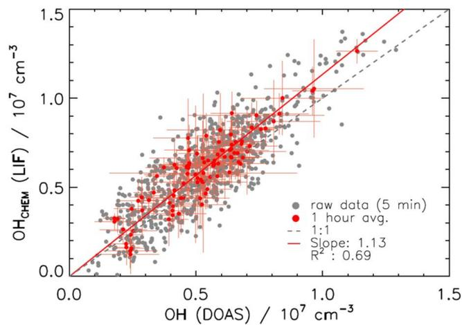
**Figure 12.** Correlation plot between OH concentrations measured by the FZI-LIF-CMR and the DOAS instruments during the summer period of the JULIAC campaign. The 814 data points are averaged over 5 minute and 1 hour. The red line is a linear fit of 5 minute data set weighted with the statistical errors of both instruments and forced to the origin. Error bars denote the  $1\sigma$  precision of the measured data
