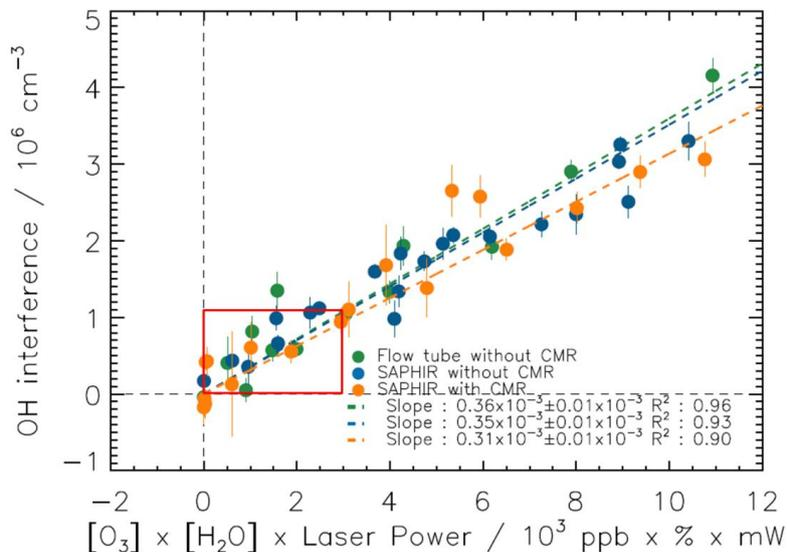
**Figure 5.** OH interference, expressed as equivalent ambient OH concentration, from the laser photolysis of ozone in humidified synthetic air for a range of concentrations of ozone, water vapour, and laser power. Tests were done with and without the CMR with a flow tube or in chamber experiments. Measurements were fitted to a linear function forced through the origin. The red box specifies the interference for concentrations of ozone and water vapour normally observed in the lower troposphere.
