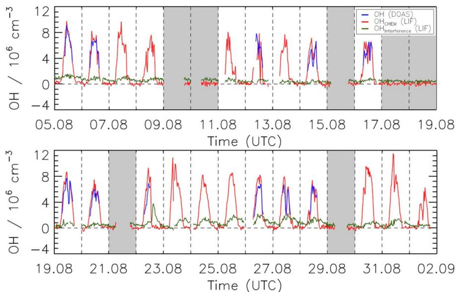
**Figure 11.** Time series of OH concentrations measured by LIF-CMR (red line) and DOAS (blue line) during the summer period of the JULIAC campaign. The green line shows the equivalent OH concentration of the interference signal in the LIF system. All data points are 30 min averages. Vertical dashed lines denote midnight. Grey shaded areas indicate when the chamber roof was closed. Data gaps occurred when measurements were stopped for calibrating instruments.
