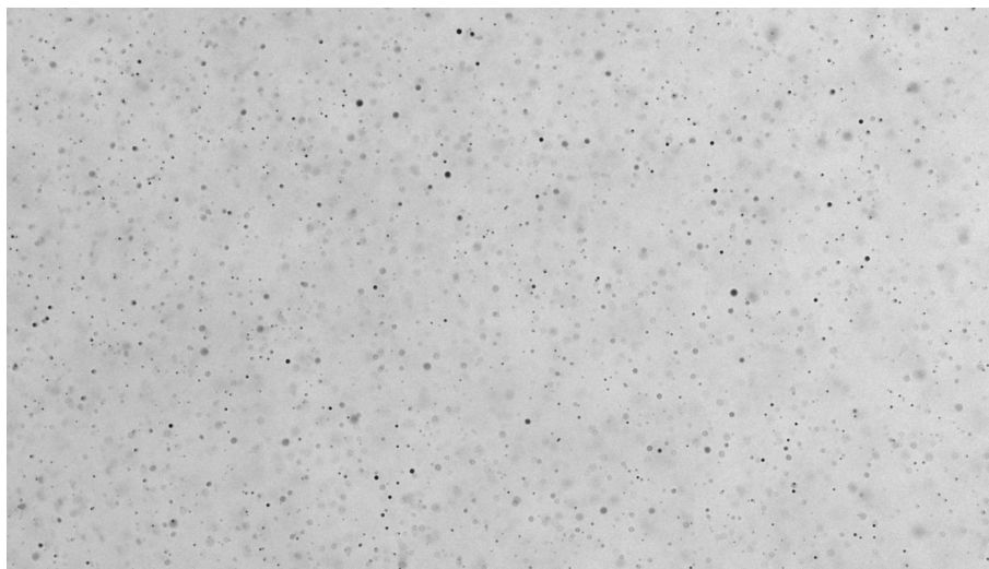
Figure 3. A typical shadow image of droplets produced by ultrasonic droplet generator taken during laboratory tests with the camera lens magnification x2.
