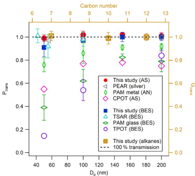
**Figure 2.** Particle (left and bottom axis) and gas (right and top axis) transmission efficiencies ( $P_{\text{trans}}$  and  $G_{\text{trans}}$ ) for the ECCC-OFR. Particle transmission efficiencies of other OFRs are shown for comparison: PAM glass and TPOT (Lambe et al., 2011), PAM metal (Karjalainen et al., 2016), TSAR (Simonen et al., 2017), CPOT (Huang et al., 2017), and PEAR (Ihalainen et al., 2019).
