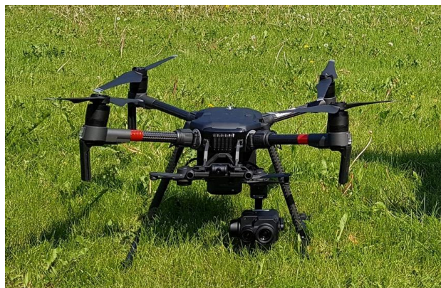
Figure 1. The UAS consisting of a drone DJI Matrice 210 v2 and a thermal/RGB camera DJI Zenmuse XT2.
