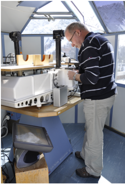
Figure 1. Illustration of the transition from manual to automated Dobson measurements. Left picture: operator in the rotating cabin with two Dobson instruments on a turntable and with an open skylight in the roof. Right: two automated Dobson instruments each on its rotating table.
