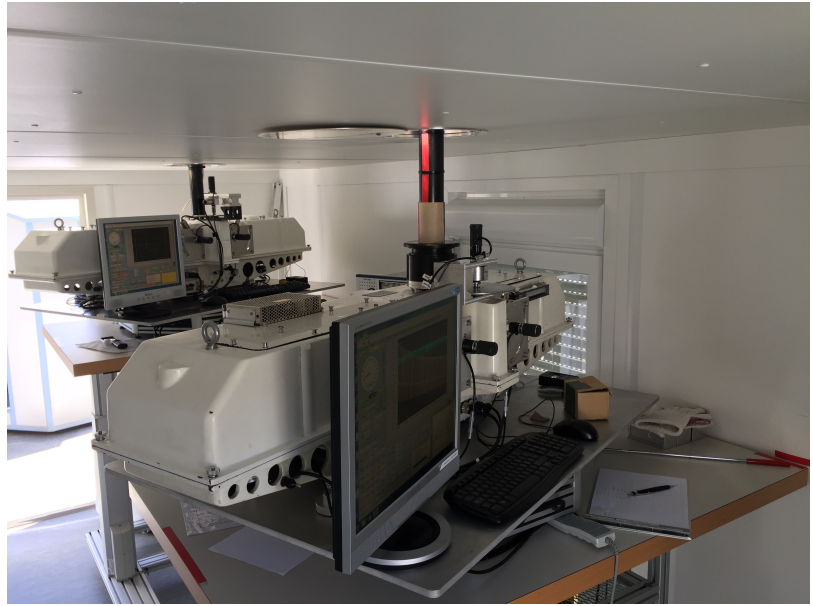
Figure 1. Illustration of the transition from manual to automated Dobson measurements. Left picture: operator in the rotating cabin with two Dobson instruments on a turntable and with an open skylight in the roof. Right: two automated Dobson instruments each on its rotating table.
