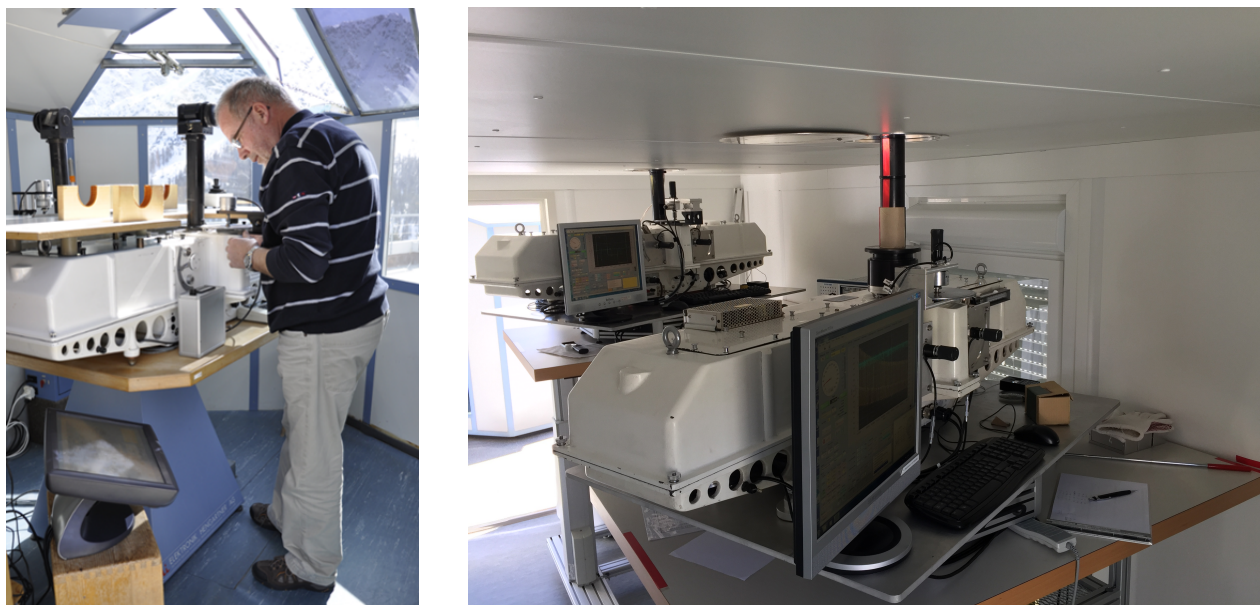
Figure 1. Illustration of the transition from manual to automated Dobson measurements. Left picture: operator in the rotating cabin with two Dobson instruments on a turntable and with an open skylight in the roof. Right: two automated Dobson instruments each on its rotating table.
