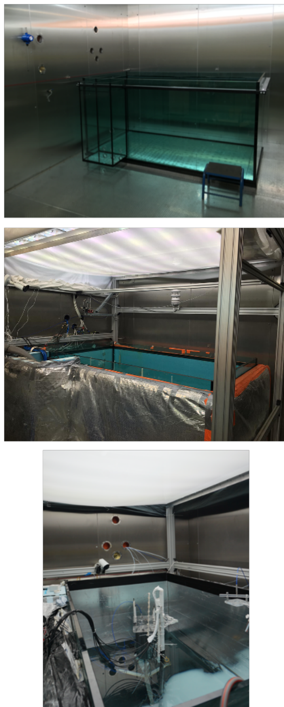
Figure 1. The tank just after installation (top), with all the main features in place (middle), and set up for experiments with visible lighting (bottom).
