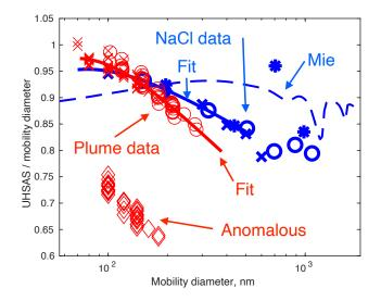
Figure 1: UHSAS sizing of NaCl in the lab tests and of plume particles in flight. The solid blue curve is a fit of the same form as used for the smoke plume particles. The dashed blue line is the Mie calculation for spherical particles with the refractive index of NaCl after correcting for the DMA mis-sizing due to non-sphericity (Zieger et al. 2017).
