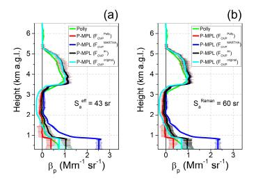
Figure 5: Dust case as observed on 29 June 2019 at 20:00-21:00 UT over Leipzig: Vertical particle backscatter coefficient (PBC),  $\beta_p$ , as retrieved in dependence of the OVP function applied to the P-MPL RCS:  $F_{OVP}$  w.r.t.
