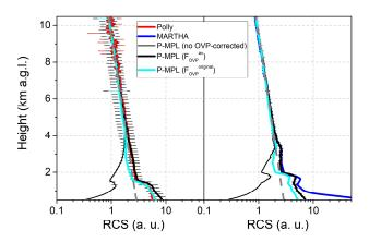
Figure 3: OVP-corrected (black thick lines) P-MPL RCS profiles by using  $F_{OVP}^{av}$  function and the uncorrected RCS ones (black thin lines), w.r.t. (Left) Polly (red line) and (Right) MARTHA (blue line) RCS profiles, together with the OVP-corrected ones by  $F_{OVP}^{original}$  (cyan lines).
