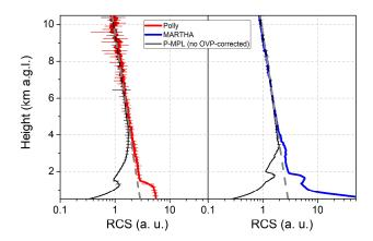
Figure 1: Comparison of the normalized (left) reference Polly (red line; for clarity, the 12 P-MPL and Polly RCS profiles, from 28 June 18UT to 29 June 05UT, were averaged) and (right) MARTHA (blue line; 4 P-MPL and MARTHA RCS profiles, from 23 July 21UT to 24 July 00UT, were averaged) w.r.t. the uncorrected by overlap P-MPL profiles (black lines). Normalization height at 9.5 km a.g.l. The aerosol-free background signal is shown by a grey dashed line.
