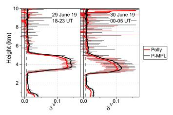
Figure 4: Volume linear depolarization ratio (VLDR),  $\delta^V$ , as obtained from both the P-MPL (black line) and Polly (15-p smoothed red line) measurements carried out on: (left) 29 June 2019, as averaged from 18 to 23 UT, and (right) 30 June 2019, as averaged from 00 to 05 UT (error bars are also shown in black and red, respectively). The aerosol-free background  $\delta^V$  is marked by a grey dashed line.
