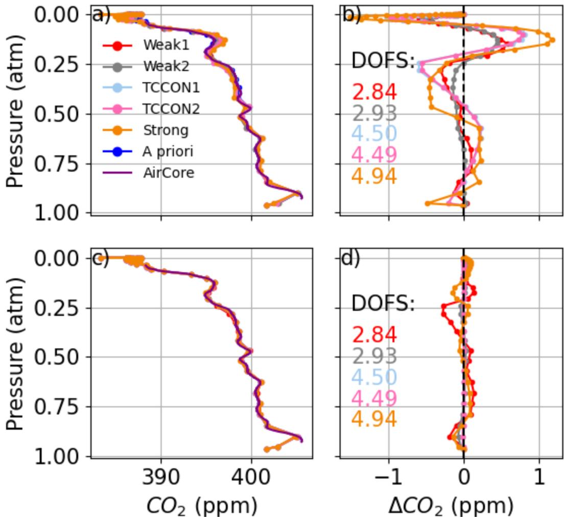
Figure R6: profiles retrieved from fits to synthetic spectra with no perturbations. In (a) with the extra convolution of the synthetic spectrum with the ILS, and in (c) without.
