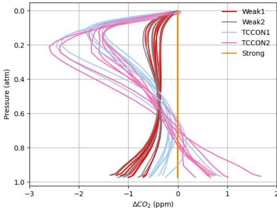
**Figure R5:** using real Lamont spectra and the AirCore profile as a priori, the zero-level offset was first retrieved from the Strong window and then added in the Weak and TCCON windows. The difference in the retrieved profiles with and without the added offset is shown for each window for all the days with AirCore profiles over Lamont. In the Strong window, where the offset is retrieved, the differences are less than 0.001 ppm.
