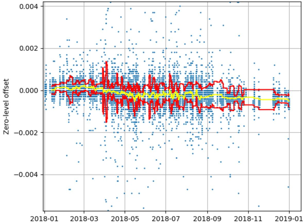
**Figure R2:** Zero-level offset retrieved from the Strong  $\text{CO}_2$  window for 1 year of measurements at the East Trout Lake TCCON station, with 52884 total spectra. The yellow line shows the 500-point rolling mean and the red lines show the 500-point standard deviation.
