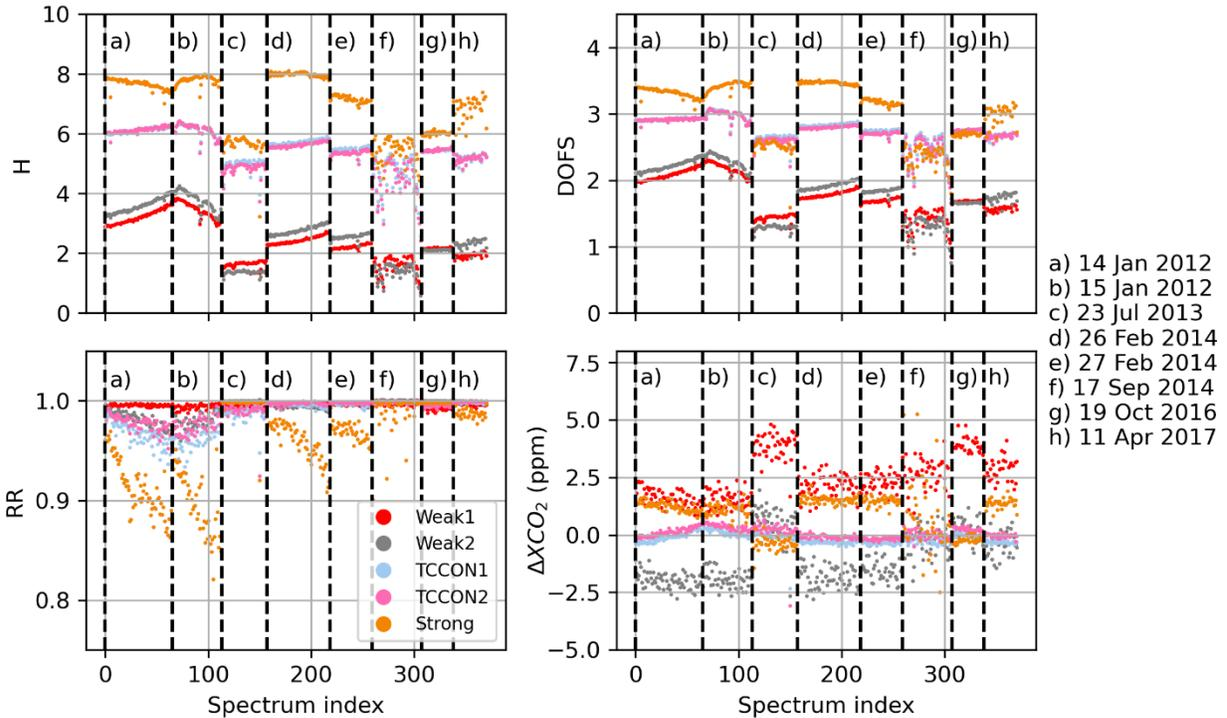
**Figure R8:** Shannon information content (top left), degrees of freedom for signal for the  $CO_2$  profile (top right), ratio of residuals (bottom left), and profile retrieval minus scaling retrieval  $XCO_2$  (bottom right), for all Lamont spectra coincident within  $\pm 1$  h of the AirCore last sampling time for AirCores launched on the dates indicated on the right, and within  $\pm 1.5$  hours of the closest GGG2020 a priori in time. Each new date is marked by a vertical dashed line.
