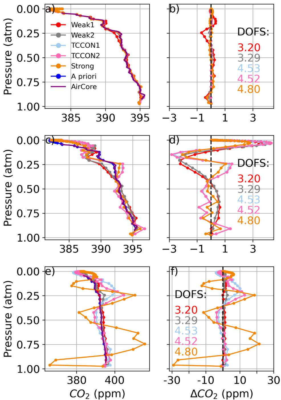
**Figure R1:** The left-hand panels show CO<sub>2</sub> profiles retrieved using synthetic spectra. In (a), we use the AirCore profile, which was used to generate the synthetic spectra, as the a priori. In (c), the field of view is perturbed by +7%, increasing the width
