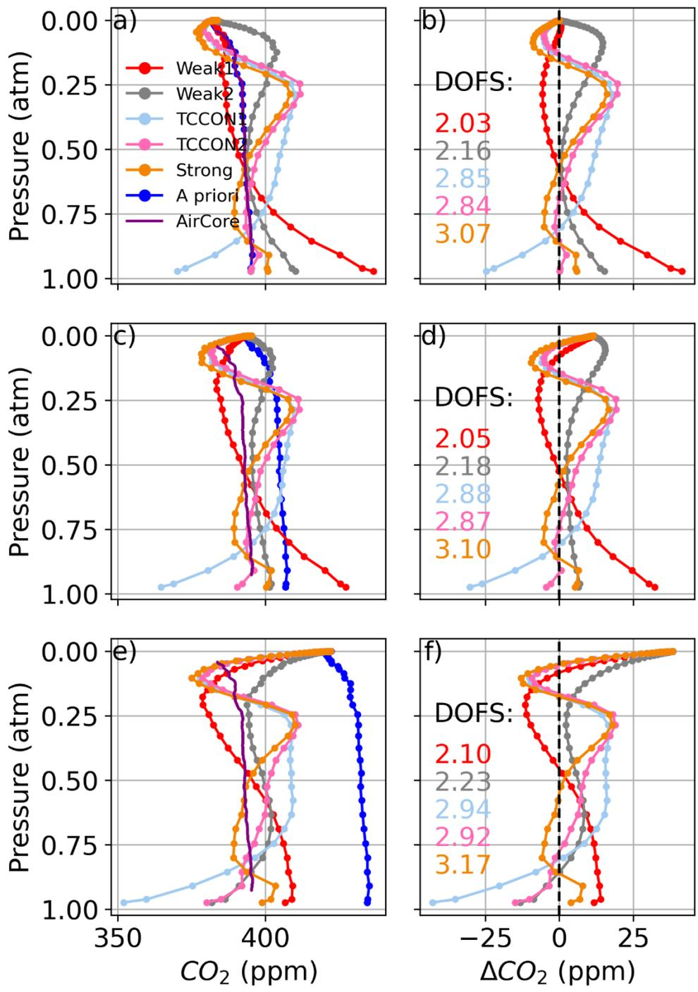
**Figure R9:** The left-hand panels show CO<sub>2</sub> profiles retrieved using real spectra on 14 January 2012. In (a), we use the AirCore profile as the a priori. In (c), the a priori is increased by 3%. In (e), the a priori is increased by +10%. The right-hand panels: (b), (d), and (f), show the difference between the retrieved profiles and AirCore, corresponding to (a), (c), and (e) respectively.
