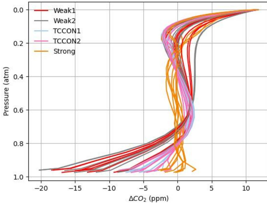
**Figure R10:** change in the profiles retrieved from real Lamont spectra when using AirCore as a priori and when using AirCore increased by 3% as a priori. Each window has 10 lines for each day with an AirCore profile over Lamont.
