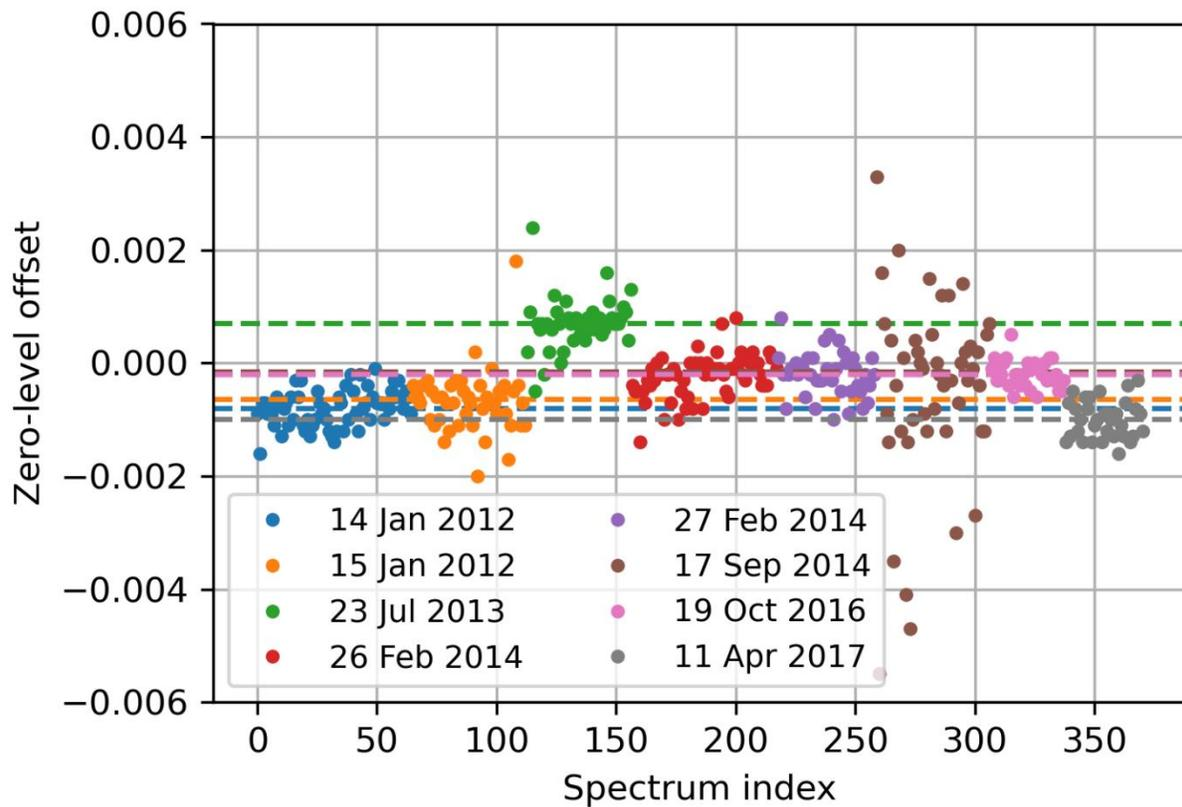
**Figure R3:** Zero-level offset retrieved from the Strong CO<sub>2</sub> window for the Lamont spectra coincident within  $\pm 1$  hour of the last AirCore sampling time and within  $\pm 1.5$  hour of the closest a priori time on each day indicated by the legend (yyyymmdd). The dashed lines represent the median value for each date.
