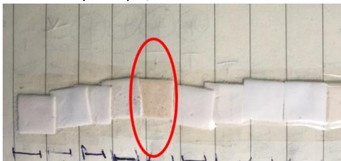
**Figure R1.** A photo of filters after OC/EC analysis. The red circle highlights an example of abundant metal oxides on the quartz filter after OC/EC analysis, leading to browning of the filter.
