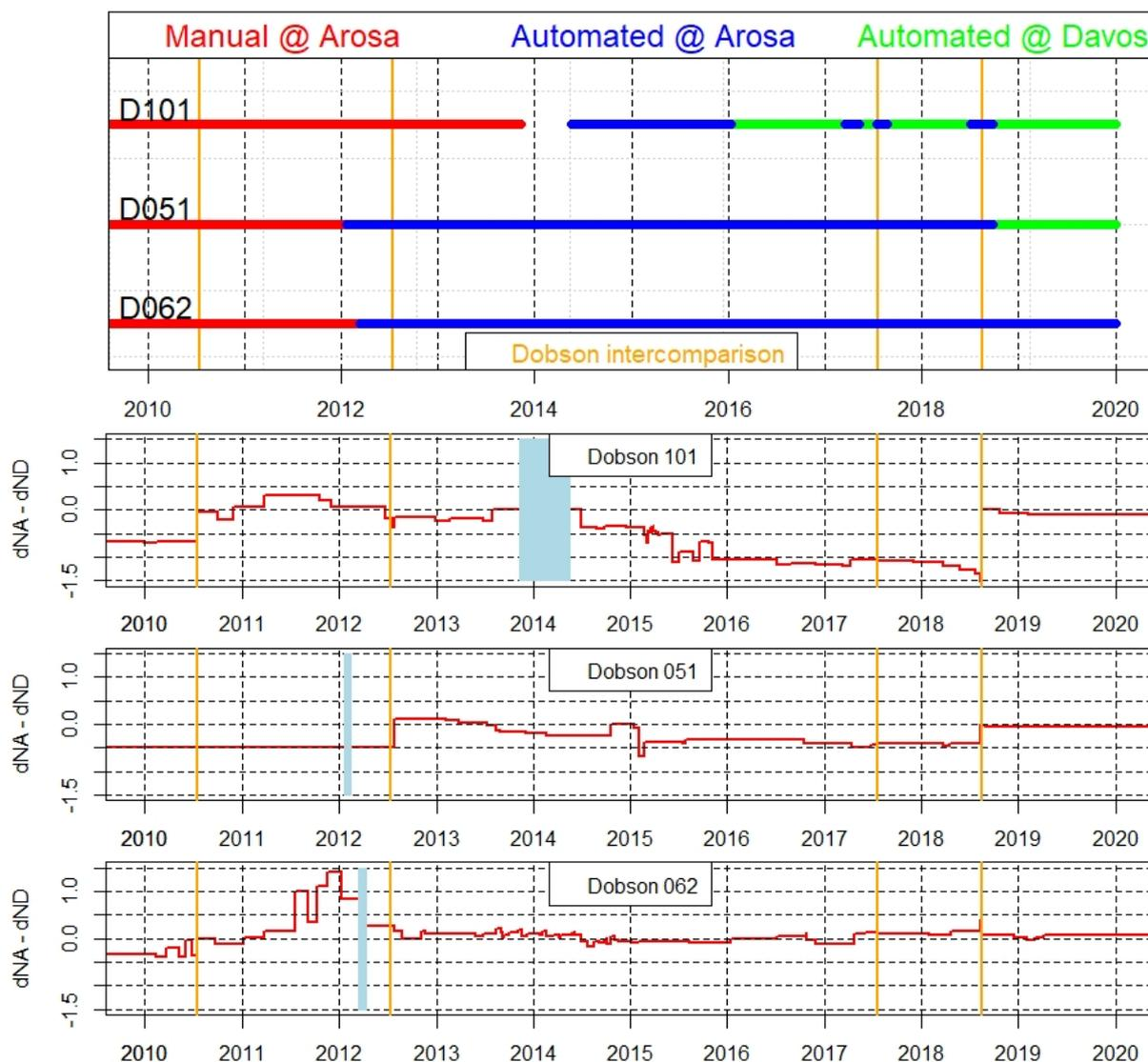
**Figure 2.** Upper panel: historical changes of the Dobson operation as well as of the instrument locations. Lower three panels : time series 2010–2020 of the lamp corrections  $\delta N_A - \delta N_D$  for the three LKO Dobson instruments. The vertical yellow bars denote the intercomparisons with the European travelling standard. The blue bands mark the unavailability of each Dobson instrument during the process of automation.
