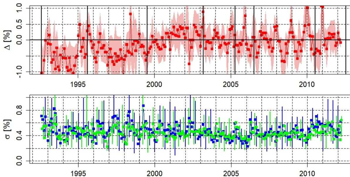
**Figure 5.** Daily analysis results: time series of the monthly median of the difference  $\Delta_{101-062} = \delta_{D_{101}} - \delta_{D_{062}}$  (upper panel) and the individual  $\sigma$  (lower panel) between coincident measurements of the Dobson instruments  $D_{101}$  and  $D_{062}$  over the period 1992–2012. Calibration campaigns are denoted by the black lines. The shading and the error bars are for the  $IP_{2.5\%-97.5\%}$  interval.
