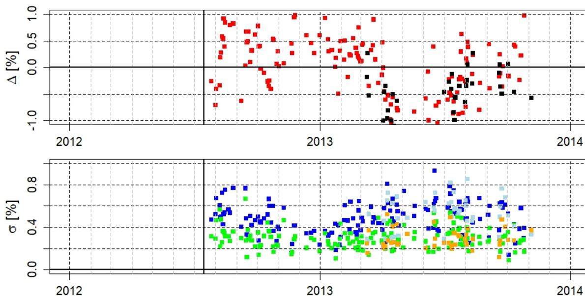
**Figure 6.** Upper panel: 2012–2013 time series of  $\Delta_{101-062}$  (red) derived from coincident measurements of  $D_{101}$  (manual) and  $D_{062}$  (automated) and  $\Delta_{101-051}$  derived from coincident measurements of  $D_{101}$  (manual) and  $D_{051}$  (automated) for 2013 (black). Lower panel: time series of  $\sigma_i$  of  $D_{101}$  (blue / light-blue),  $D_{062}$  (green) and  $D_{051}$  (orange).
