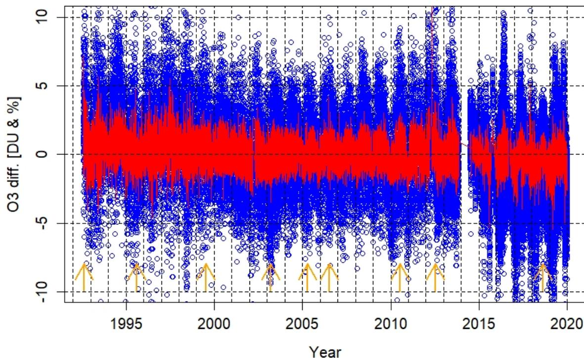
**Figure 3.** Time series of the differences between individual coincident measurements of the Dobson instruments  $D_{101}$  and  $D_{062}$  over the period 1992–2019. Blue: difference  $D_{062} - D_{101}$  in Dobson units [DU]. Red: difference  $D_{062} - D_{101} / D_{101}$  in [%]. Yellow arrows indicate the calibration / maintenance campaigns.
