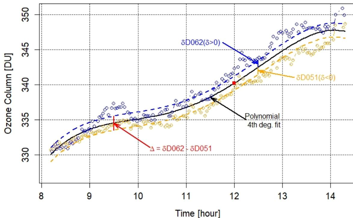
**Figure 4.** Illustration of the daily values of coincident  $D_{062}$  and  $D_{051}$  automated Dobson measurements for March 27 2016. The black line is the polynomial fit and the dashed lines correspond to the bias  $\delta_{D062}$  of  $D_{062}$  data (blue), respectively the bias  $\delta_{D051}$  of  $D_{051}$  data (orange). The difference,  $\Delta_{062-051}$  (red), is the bias between  $D_{062}$  and  $D_{051}$  instruments evaluated from the coincident measurements of that day.
