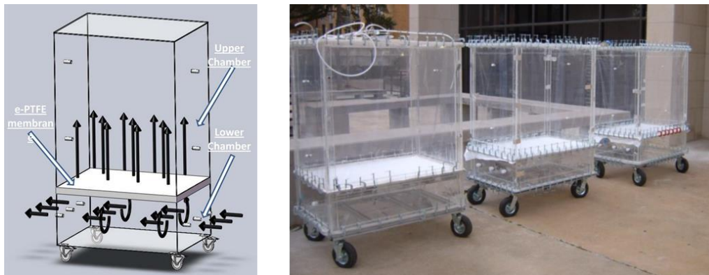
Figure S1. First generation CAGE chambers, which were referred to as QUALITY chambers in some publications.
