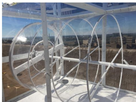
25 Figure S2. Close-up photo of a CAGE chamber highlighting the overall clarity.
