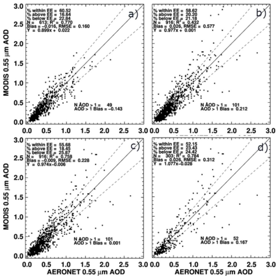
820 Figure 9 Comparisons of the MODIS DT AOD at 0.55 μm against collocated AERONET observations during January, February, and March 2013 over China. a) Operational DT AOD, b) an intermediate AOD retrieved using the same LUT as the operational DT but with modified masking, c) AOD retrieved with the full regional research algorithm, and d) the extra collocations that are in c) but not in a).
