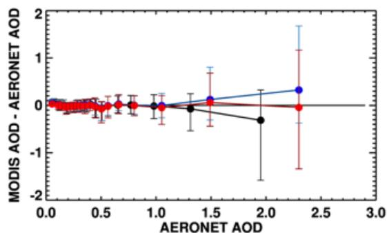
825 Figure 10 Bias between MODIS and AERONET over land AOD at 0.55 μm as function of AERONET AOD at 0.55 μm. Black represents the operational DT AOD, blue represents the AOD using the operational LUT but with new masks, and red represents
