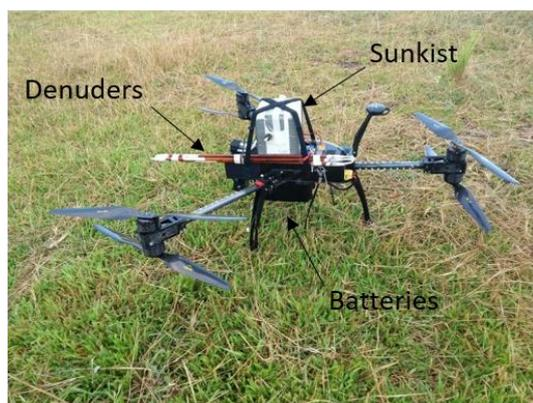
505 **Figure 5: Drone-based denuder sampling setup and SO<sub>2</sub> sensor (Sunkist)**
