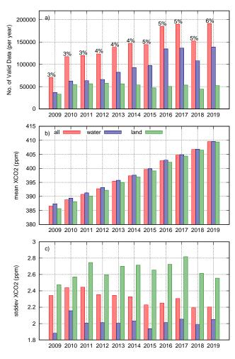
**Figure 17.** Statistics for valid GOSAT measurements (after pre- and post-processing filtering) for each year. Blue: Measurements over water. Green: Measurements over land. Red: All data. a) Number of valid measurements, incl. percentage of all originally available measurements. b) Global mean  $XCO_2$ . c) Corresponding standard deviation.
