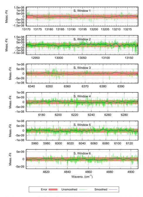
Figure 13. GOSAT residuals (measurement - fit) for data from Fig. 9 (S polarisation). Green: Unsmoothed. Blue: Smoothed with a boxcar of width 21 spectral pixels (=  $4.2 \, \mathrm{cm}^{-1}$ ). Red: Estimated noise error range. Radiance difference unit is  $\mathrm{W/cm}^2/\mathrm{cm}^{-1}/\mathrm{sr}$ .
