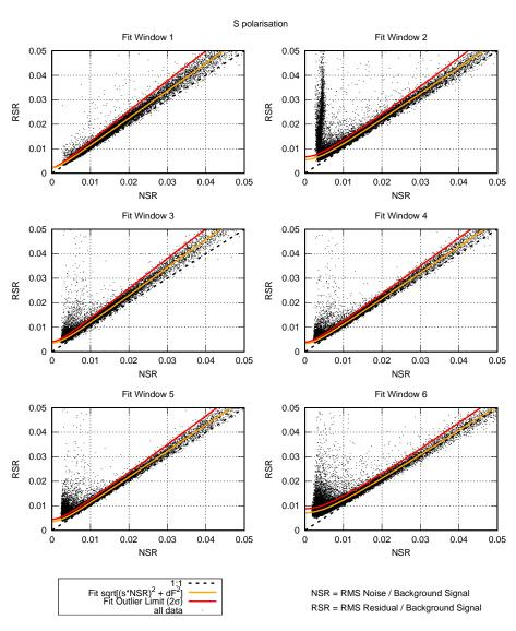
Figure 3. GOSAT noise model (S polarisation).
