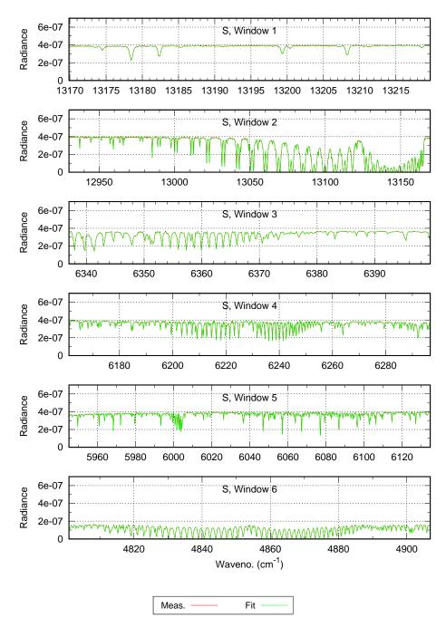
Figure 9. Example for a single GOSAT measurement (S polarisation): Measured (red) and retrieved (green) spectra in the different fit windows; because of the good agreement the red curve is essentially barely visible below the green curve. Radiance unit is  $W/cm^2/cm^{-1}/sr$ .
