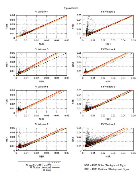
Figure 6. GOSAT-2 noise model (P polarisation).
