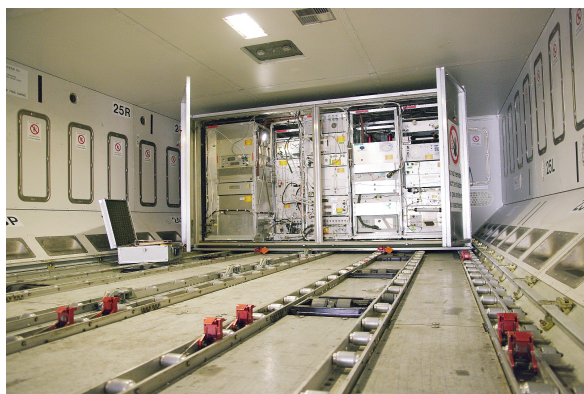
Figure 5. Picture of the CARIBIC laboratory container (1.65 tons, 19 instruments in 2017) inside the aircraft cargo bay.
