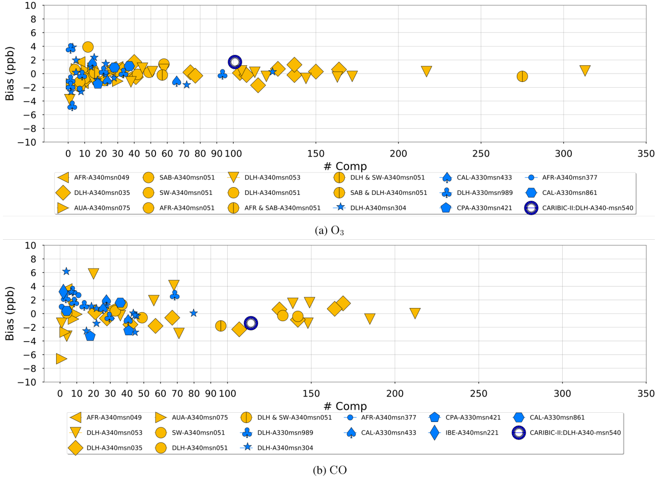
Figure 11. Dependency of the O 3 (a) and CO (b) instrument measurement mean bias for each FP with the number of flight inter-comparison profiles. Different symbols are used for each distinct aircraft (same as Figure 10), the yellow color is for the MOZAIC program and the blue color is for IAGOS and CARIBIC.
