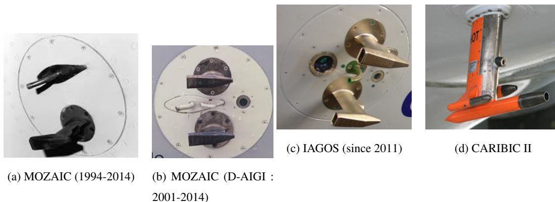
Figure 3. Pictures of the inlet plates used throughout the various programs. In a), b) and c), air for O_3 and CO measurements is collected through the small facing forward pitot tube. In c), it is done using the lowest small inlet. Other inlets and Rosemount pitots are for water, aerosol or other gases measurements. The inlet shown in b) was installed on 1 MOZAIC aircraft (D-AIGI) with an additional Rosemount inlet for NO_y/NO_x measurements. It is the precursor of the IAGOS inlet.
