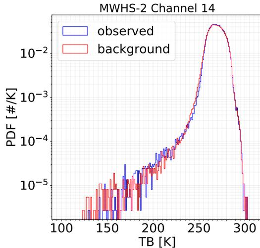
**Figure 1.** Probability distribution functions (PDFs) of simulated and observed brightness temperatures for MWS-2 channel 14. The data covers latitude range  $60^\circ$  S to  $60^\circ$  N, and satellite zenith angle less than  $7.5^\circ$ .
