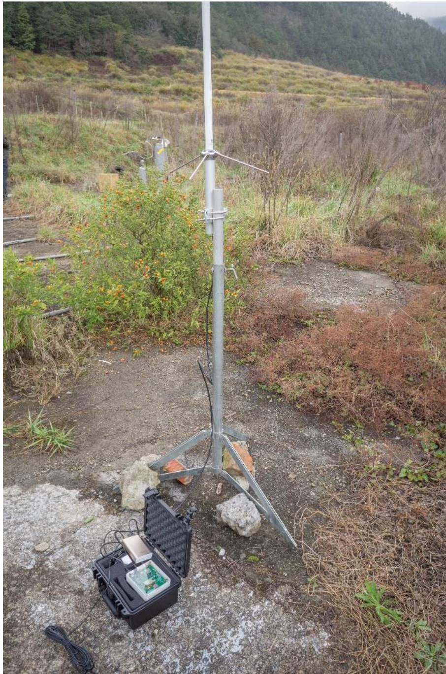
468 Figure 7. A typical setup of the ground receiver in the field, with the 433Mhz antenna in 469 the middle, and the receiver, GPS antenna and power bank at the bottom black box.
