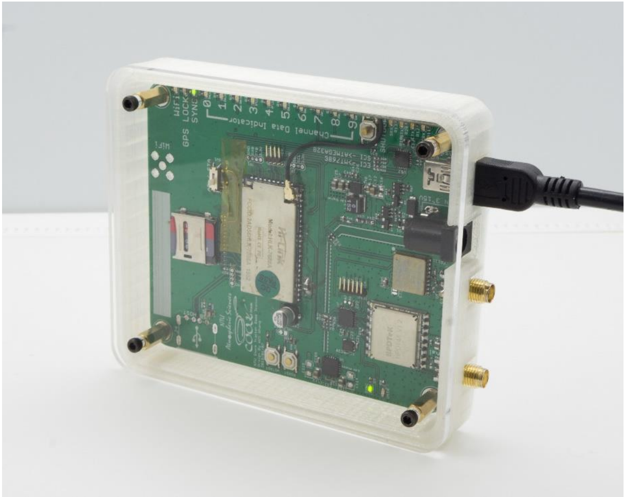
459 Figure 6. Photo of a Storm Tracker Ground Receiver. On the right are the GPS module 460 and RF module to receive the signal, along with the USB and DC power jack for power 461 input and the console access. In the middle is the central processor, which handles data 462 recording and hosts the website. On the left is the SD card for storage. On the top are the 463 indicator LEDs, which show the current status of the receiver and the received data 464 channels.
