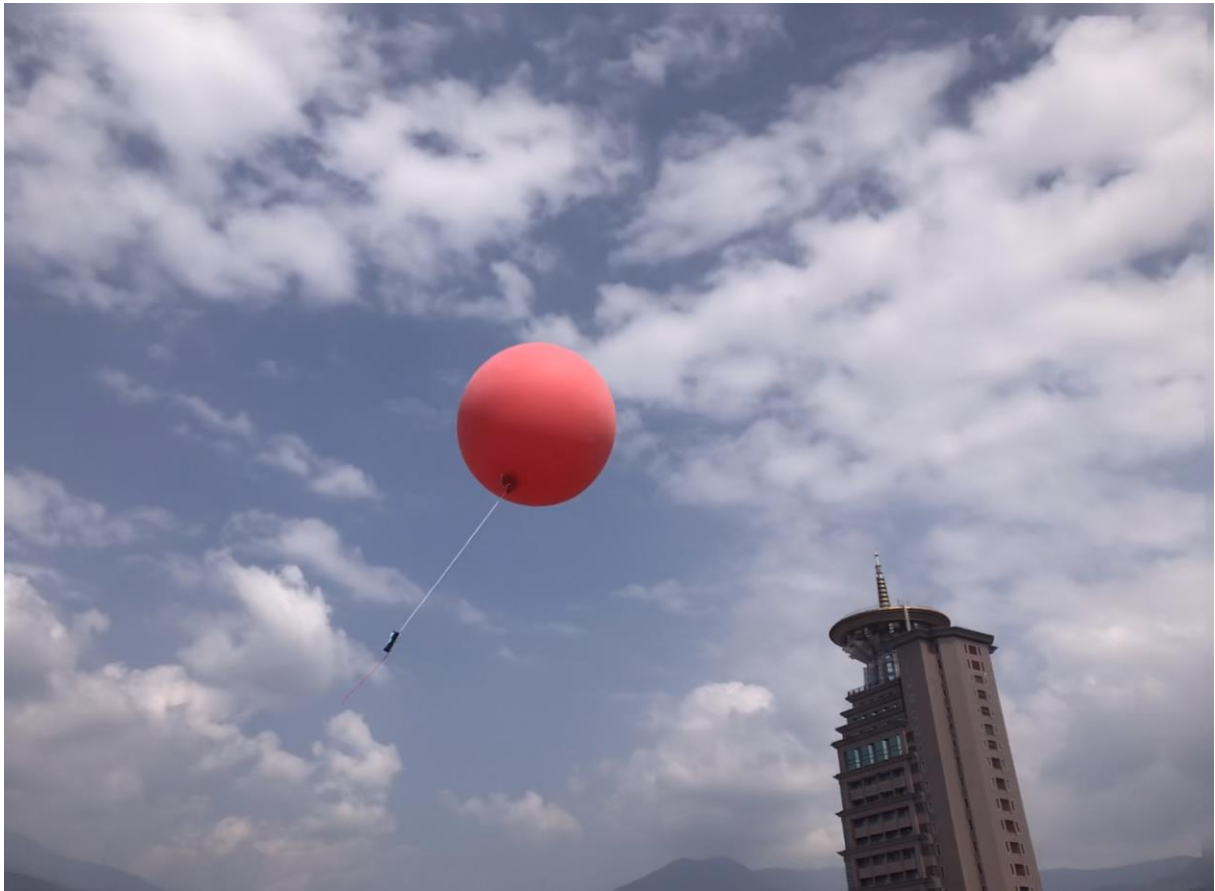
454 Figure 5. A Storm Tracker (without enclosure) launched with a pilot rubber balloon (20g) 455 during a field campaign.
