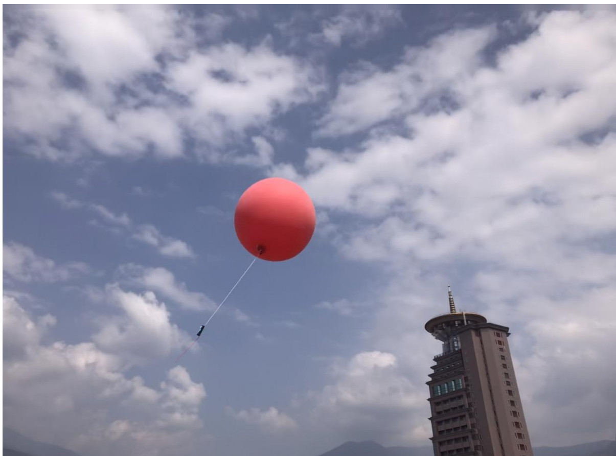
490 Figure 5. A Storm Tracker (without enclosure) launched with a pilot rubber balloon (20g) 491 during a field campaign.
