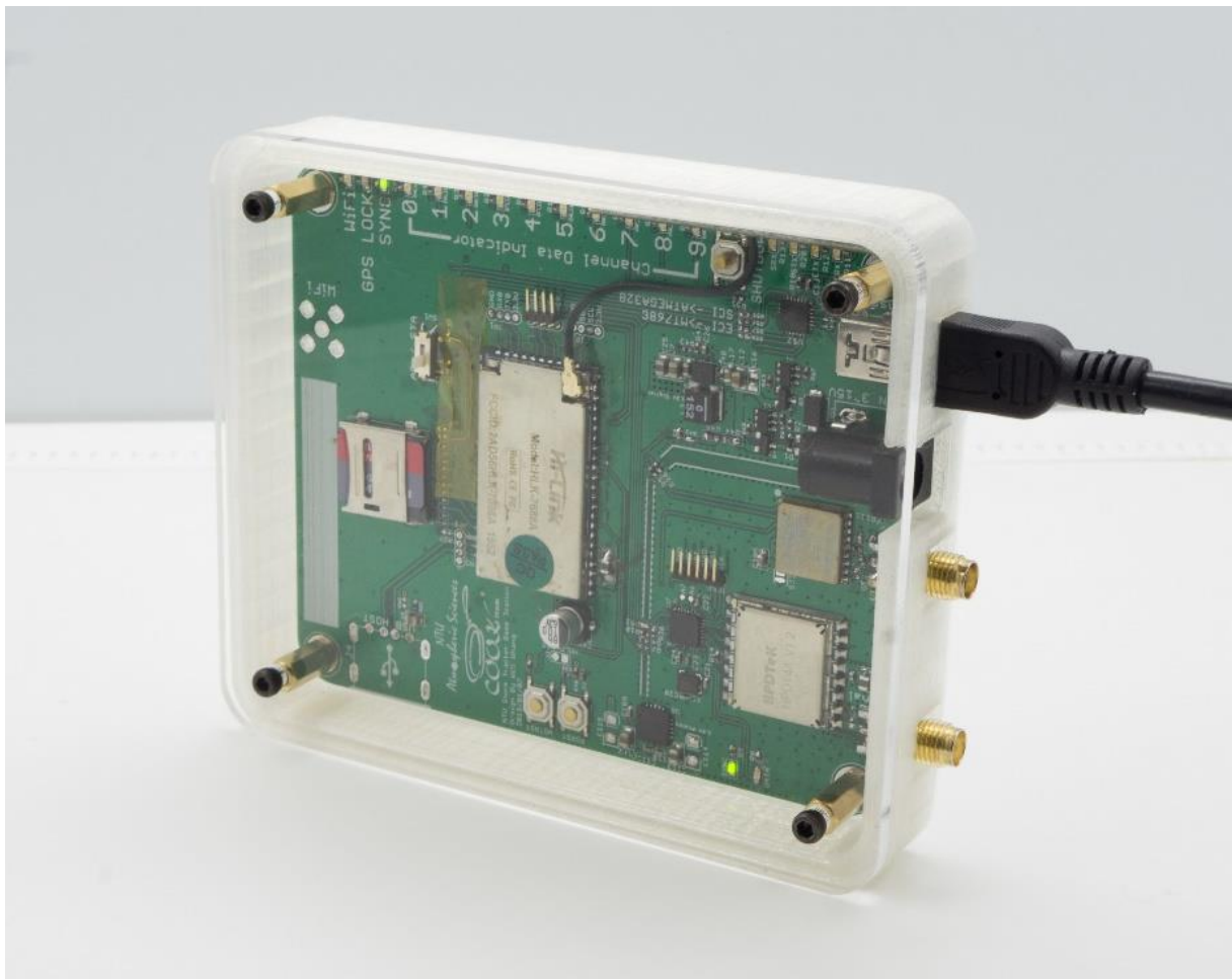
495 Figure 6. Photo of a Storm Tracker Ground Receiver. On the right are the GPS module 496 and RF module to receive the signal, along with the USB and DC power jack for power 497 input and the console access. In the middle is the central processor, which handles data 498 recording and hosts the website. On the left is the SD card for storage. On the top are the 499 indicator LEDs, which show the current status of the receiver and the received data 500 channels.
