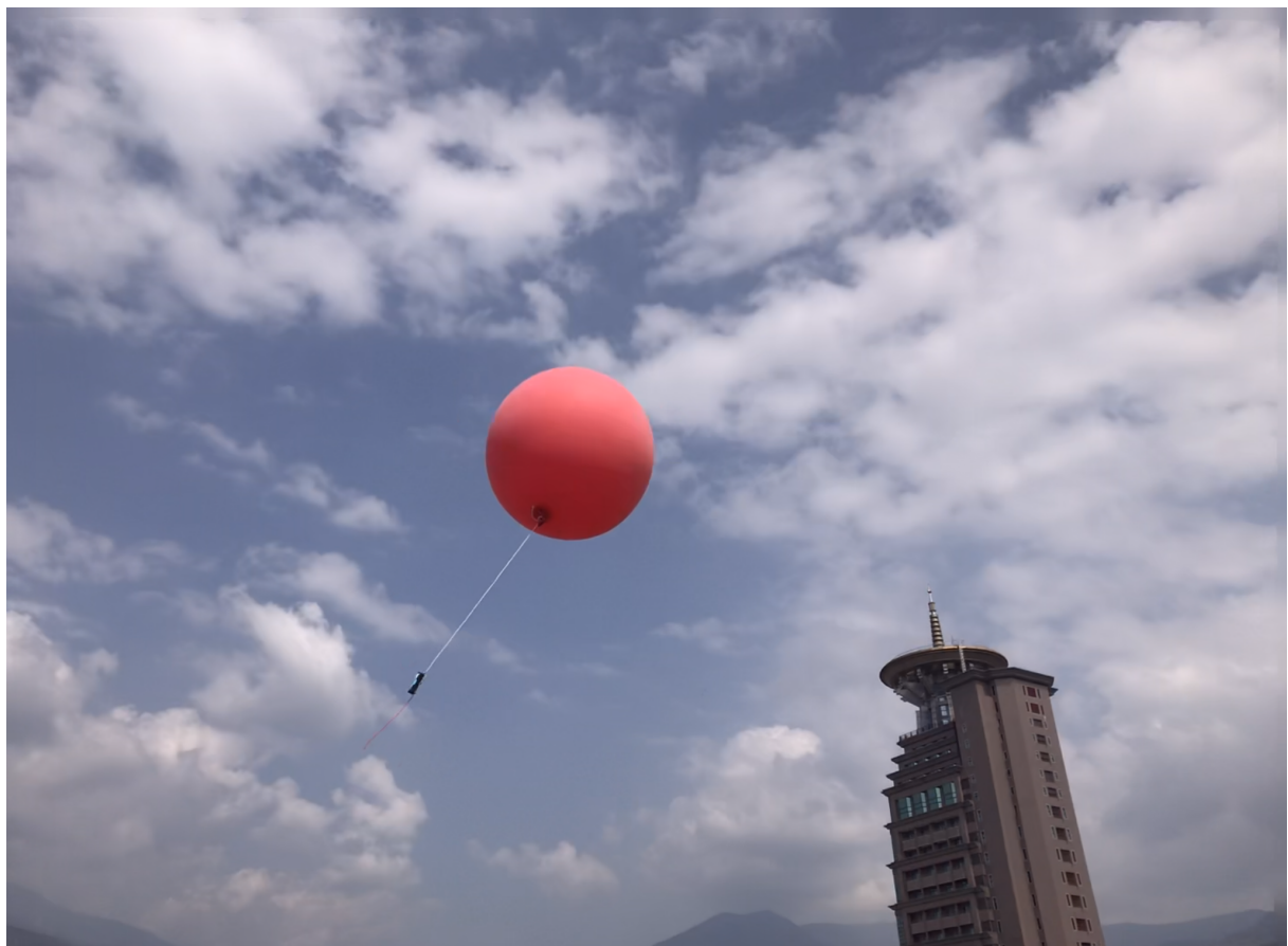
453 Figure 5. A Storm Tracker (without enclosure) launched with a pilot rubber balloon (20g) 454 during a field campaign.
