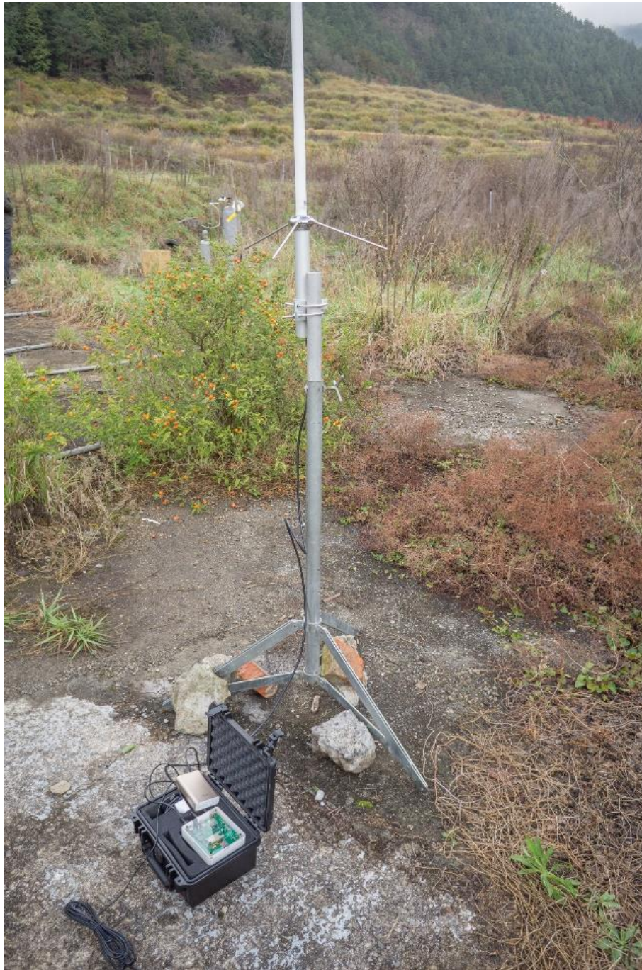
Figure 7. A typical setup of the ground receiver in the field, with the 433Mhz antenna in the middle, and the receiver, GPS antenna and power bank at the bottom black box.
