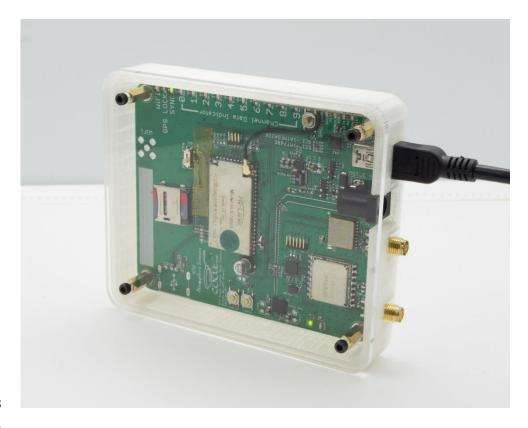
Figure 5. Photo of a Storm Tracker Ground Receiver. On the right are the GPS module and RF module to receive the signal, along with the USB and DC power jack for power input and the console access. In the middle is the central processor, which handles data recording and hosts the website. On the left is the SD card for storage. On the top are the indicator LEDs, which show the current status of the receiver and the received data channels.
