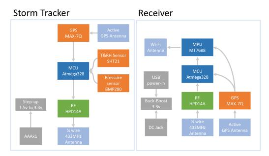
Figure 1. System block diagram for the Storm Tracker system, including Storm Tracker (left) and Receiver (right). The part number for the chipset is indicated in the box, and the arrow indicated the dataflow.
