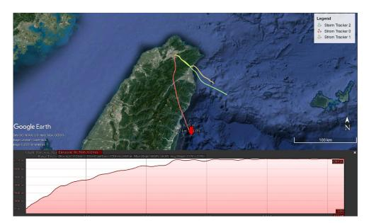
Figure 15. Three balloon tracks during Typhoon Talim (top) and the height profile of the Strom Tracker 0 (bottom). The launching site is located on campus of the National Taiwan University. The maximum range of the Storm Tracker from the site is 132km, in which the Storm Tracker could maintain at about 6200m height. Credit to © Google Earth Pro for providing the satellite image.
